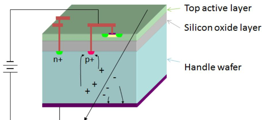
**Figure 1.** SOI wafer used as a monolithic detector. A sensor is created in the bottom handle layer and connected to the readout in the active layer with metal vias.
