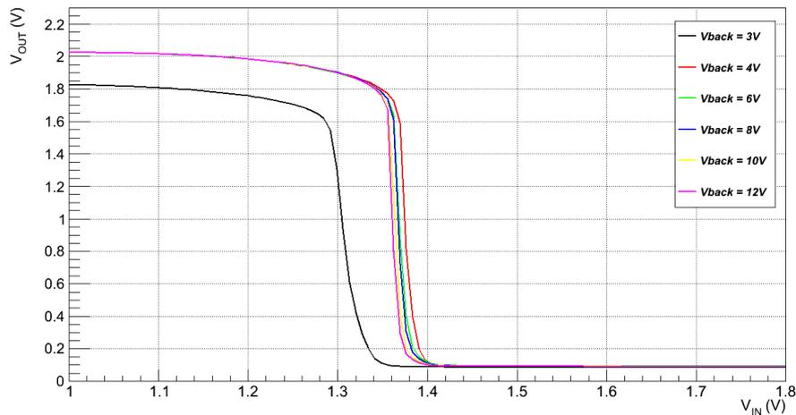
**Figure 6.** 3T transfer curve with varying back voltage.
