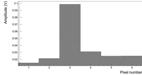
**Figure 13.** Amplifier pixel output with laser targeted on Pixel 3.
