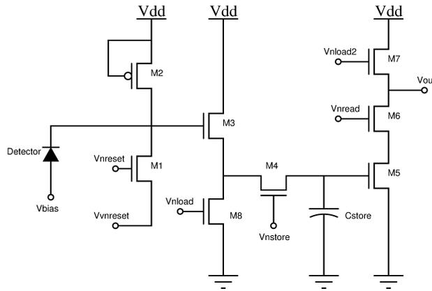
**Figure 5.** 3T readout circuit with storage capacitor.
