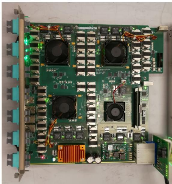
**Figure 7.** Fully assembled gFEX prototype v3 board. There are four large FPGAs and 35 MiniPODs, and it is a 2-slot module.
