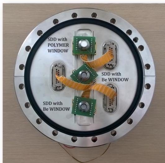
**Figure 3.** Photo of the vacuum flange with mounted detectors.
