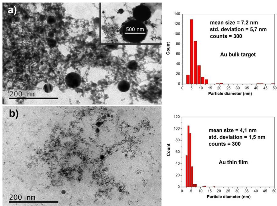
**Figure 1.** TEM images and corresponding histograms of the particles size distribution of Au nanoparticles produced by laser ablation of Au bulk target (a) and Au thin film (b) in water.
