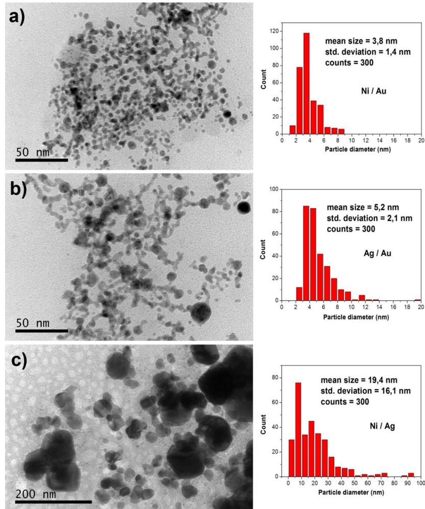
**Figure 3.** TEM images and corresponding size distribution histograms of nanoparticles produced by laser ablation in water of multicomponent thin films: Ni/Au (a), Ag/Au (b) and Ni/Ag (c). The ablation is performed by using laser wavelength of 355 nm and laser fluence of  $5 \text{ J/cm}^2$ .
