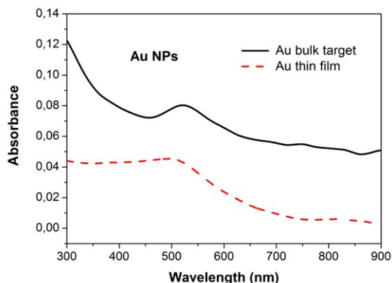
**Figure 2.** Optical absorption spectra of colloids produced by laser ablation of Au bulk target and Au thin film in water at laser wavelength of 355 nm and laser fluence of 5 J/cm<sup>2</sup>.
