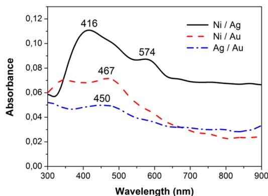
**Figure 4.** Optical absorption spectra of colloids produced by laser ablation of multicomponent (Ni/Ag, Ni/Au, and Ag/Au) thin films in water at the laser wavelength of 355 nm and laser fluence of  $5 \text{ J/cm}^2$ .
