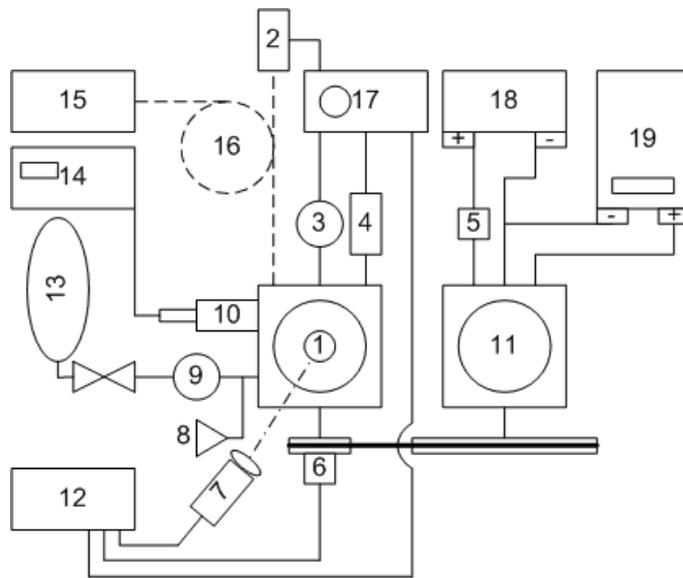
**Figure 1.** Experimental setup: 1—engine; 2—photomultiplier tube; 3—pressure sensor; 4—temperature sensor; 5—regulation relay; 6—rotation sensor; 7—laser; 8—drop oilier; 9—flow rate sensor; 10—silencer; 11—dc generator; 12—synchropulse generator; 13—gas bottle; 14—gas analyser; 15—spectrometer; 16—optical fiber; 17—oscilloscope; 18—accumulator; 19—electronic load.
