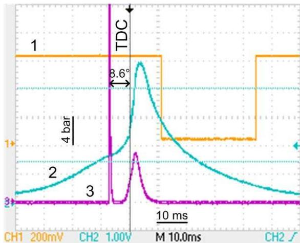
**Figure 2.** Typical oscillogram at 2.2 Hz: 1—rotation encoder; 2—pressure sensor (0.25 V/bar); 3—radiation sensor.
