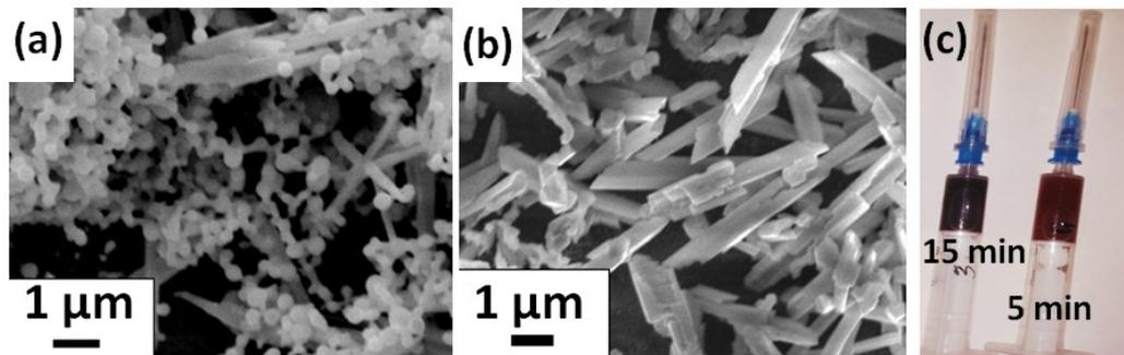
**Figure 6.** SEM-images of dried Se NRs deposits on silica-supported Ag films with 5 min (a) and 15 min (b) laser exposition of Se target; (c) – a photograph of the corresponding Se-colloids in medical syringes.
