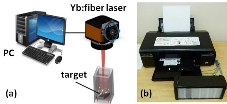
**Figure 1.** (a) – experimental setup for nanoinks fabrication; (b) – inkjet printer Epson L800.
