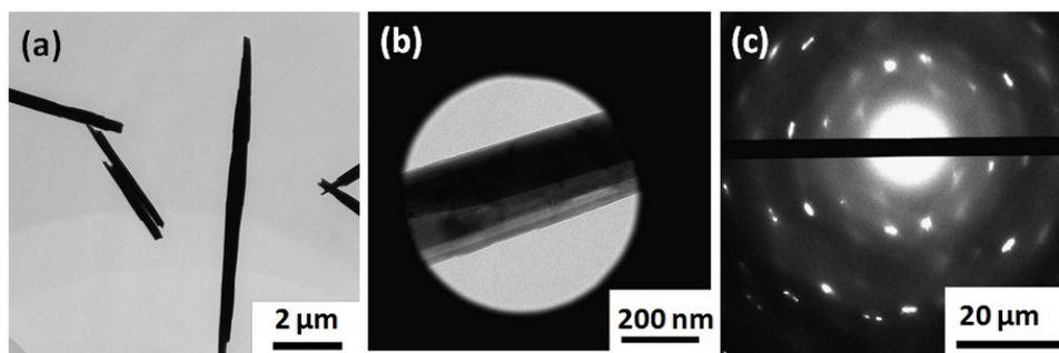
**Figure 4.** TEM-photographs of Se nanorods (a), (b) and the corresponding electron diffraction pattern (c).
