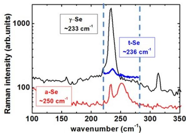
**Figure 3.** Raman spectra of solid  $\gamma$ -Se (black curve), amorphous a-Se NPs (red curve) and trigonal t-Se nanorods (blue curve).
