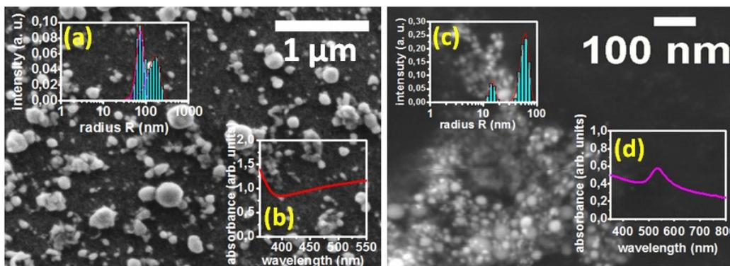
**Figure 2.** SEM-images of Se (left) and Au (right) NPs, printed on silica-supported silver films. Insets: (a), (c) – the corresponding DLS spectra of NPs size distribution; absorbance spectra of Se NPs (b) and Au NPs (d).
