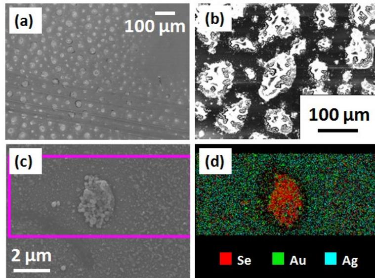
**Figure 5.** SEM-images of inkjet printed multilayers of Se and Au NPs on the silica-supported Ag film (a), (b), (c) and the corresponding EDS-map (d): Se 0.79 at. %; Au 0.38 at. %; Ag 7.69 at. %.
