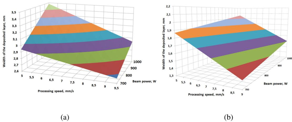
**Figure 1.** The dependence of the width of the cushion from the factors of the experiment (a - scanning, b – without scanning).
