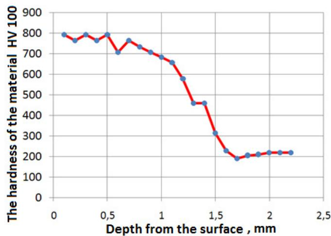
**Figure 2.** The dependence of micro-hardness on the depth.
