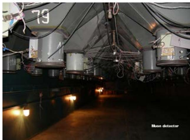
**Figure 2.** First stage of the Muon Detector, 175m<sup>2</sup>, in operation since 1999.
