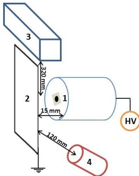
**Figure 2.** The scheme for testing the neutron generator on nanotubes. 1- duralumin holder with fixed silicon substrate with CNT array, 2 - target with deuterated film, 3 -  $^3\text{He}$  counter, 4 - neutron scintillation spectrometer.
