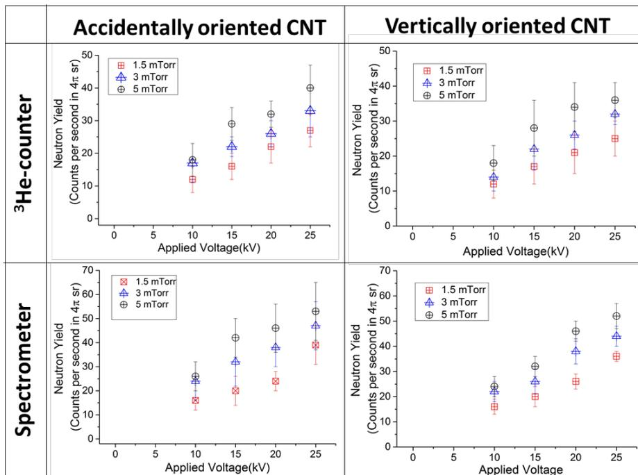
**Figure 3.** Dependence of the neutron yield on the residual gas pressure and the applied potential for two different types of CNT arrays, which measured using  $^3\text{He}$  counter and scintillation spectrometer.
