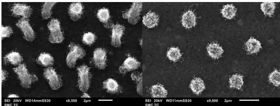
**Figure 1.** Image of fragments of the array of carbon nanotubes on Si substrate, obtained by scanning electron microscope (Performed in the NME RAS). Right - CNT with vertical orientation, left - with accidental orientation.
