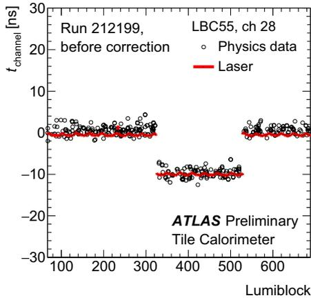
**Figure 2.** Example of sudden change in the time calibration as detected by the laser-based tool in one channel [6]. Superimposed are the results obtained with the jet collision data.
