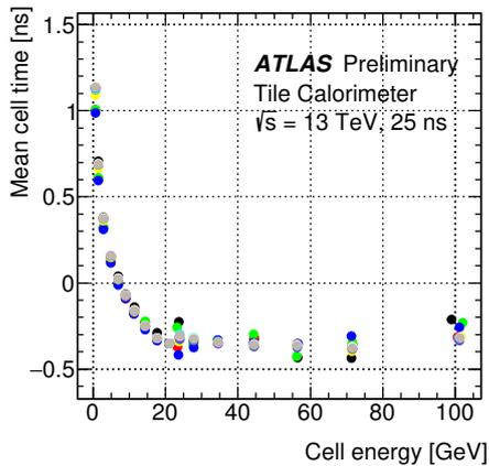
**Figure 4.** The mean cell time as measured with jet collision data as a function of energy deposited in the cell, after correcting for the run-to-run differences [6]. Symbols of different colours correspond to different runs.
