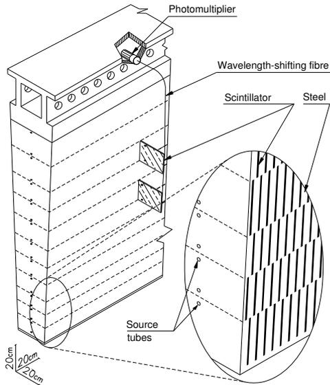
**Figure 1.** The sketch of one TileCal module shows its geometry and the principle of the signal readout [2]. The scintillating tiles are oriented parallel to the incoming particles. They are readout on both edges by wavelength-shifting (WLS) fibers, which route the light to the photomultipliers (PMTs) housed in the outer part together with the front-end electronics. The readout cells are defined by grouping the fibers onto a PMT.
