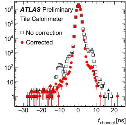
**Figure 3.** The impact of the time constant corrections for sudden changes in the time calibration, as observed for one data-taking period in Run-1 [6]. The RMS of the measured time distribution improves from 0.90 ns to 0.82 ns.
