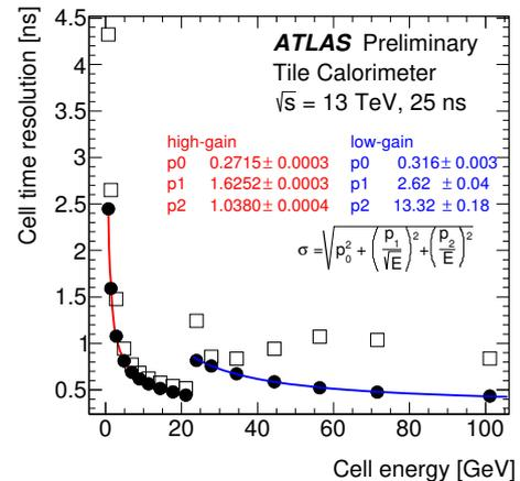
**Figure 5.** The cell time resolution as measured with jets [6]. Full circles denote Gaussian widths and open squares indicate the RMS of the underlying time spectra. The discontinuity around 25 GeV corresponds to the transition between the high- and low-gain.
