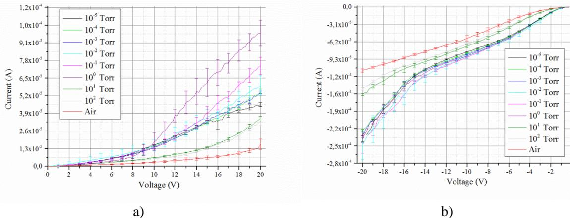
**Figure 3.** The CVC of the prototype at different pressures with a) positive and b) negative voltage polarity.
