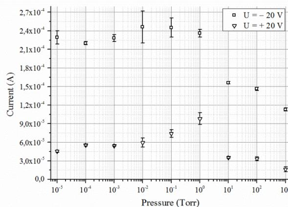
**Figure 4.** The dependence of the current on the pressure at different voltages applied to the electrode with CNTs.
