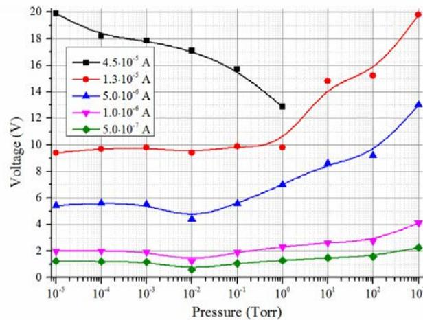
**Figure 5.** The dependence of the voltage on the chamber pressure at various currents.
