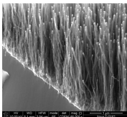
**Figure 2.** The CNT array grown on the lower electrode.
