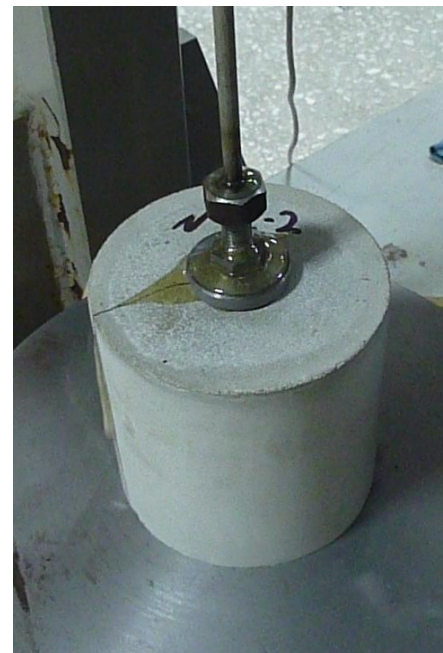
Figure 1. Destroyed sample and the loading system.
