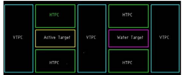
Figure 2. Schematic view of the new design under study for the ND280 upgrade. VTPC (HTPC) stands for vertical (horizontal) TPC.
