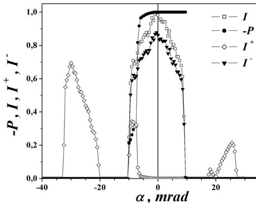
**Figure 5.** Calculated dependencies on angle  $\alpha$  (see Figs. 2 and 3) of normalized intensities  $I^+$  and  $I^-$  for, respectively, (+) and (-) spin components of monochromatic neutron beam with  $\lambda = 5.5 \text{ \AA}$  transmitted through the first polarizer. Dependencies on  $\alpha$  are also shown of intensity at the entrance of the polarizer  $I$  and polarization  $P$  of the transmitted beam.
