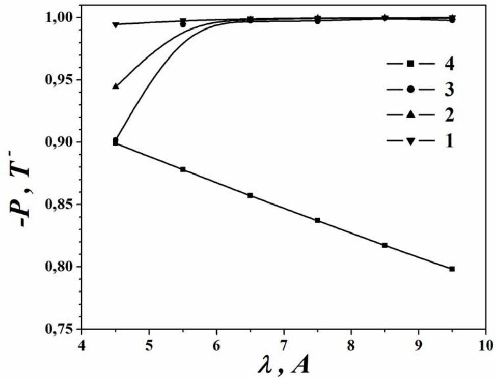
**Figure 7.** Calculated wavelength dependencies of polarization  $P$  (curves 1-3) and transmission coefficient  $T^-$  (curve 4) (in which the absorption in silicon is taken into account) of neutrons of (-) spin component (curve 4) for the beam transmitted through the first polarizer. Curves 1, 2 and 3 are obtained for angular divergences of the beam at the exit of polarizer of 8 mrad ( $\pm 4$  mrad), 10 mrad ( $\pm 5$  mrad) and 12 mrad ( $\pm 6$  mrad), respectively.
