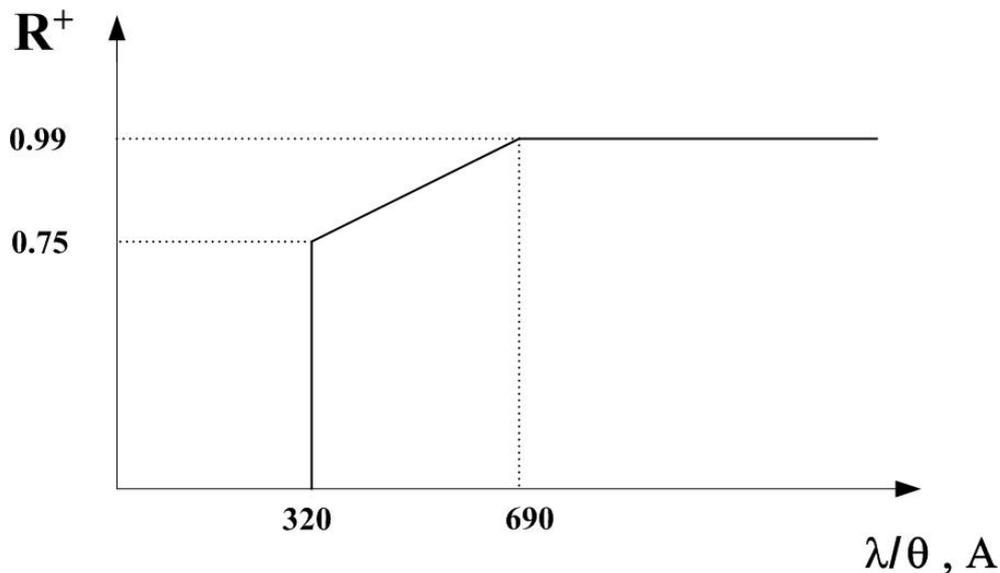
**Figure 4.** Modeling reflection coefficient of spin-up neutrons from supermirror polarizing coating  $CoFe/TiZr$  ( $m = 1.81$ ) evaporated on polished silicon substrates for reflection from silicon in dependence of parameter  $\lambda/\theta$ .
