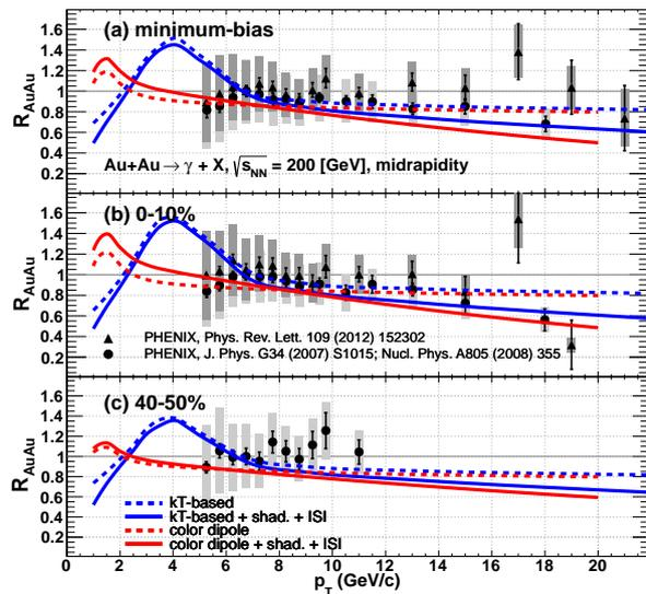
**Figure 3.** Comparison of the PHENIX data on  $R_{AuAu}$  [5] at midrapidity and for several centralities with the model based on  $k_T$  factorization (blue line) and with calculations based on the color dipole formalism (red lines). The solid and dashed lines represent calculations with and without ISI effects.
