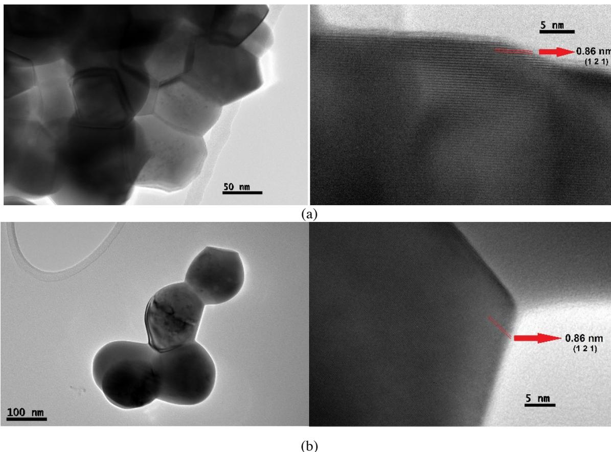
**Figure 4.** TEM images of interplanar distance and average particle size of (a)  $\text{LaCr}_{0.8}\text{Fe}_{0.2}\text{O}_3$  and (b)  $\text{LaCr}_{0.6}\text{Co}_{0.2}\text{Fe}_{0.2}\text{O}_3$ .
