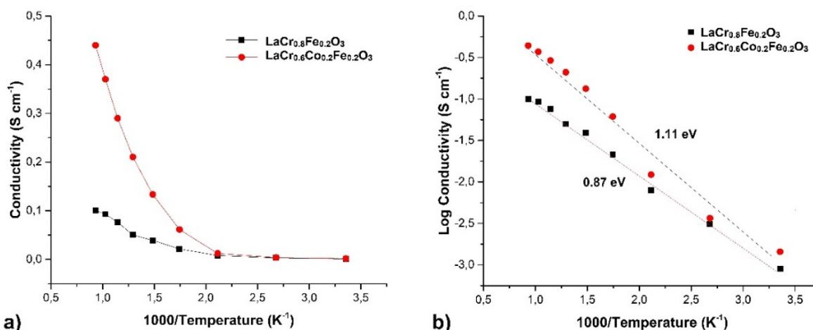
**Figure 6.** (a) Plot of conductivity and (b) Arrhenius plot from 25 °C to 800 °C of  $\text{LaCr}_{0.8}\text{Fe}_{0.2}\text{O}_3$  and  $\text{LaCr}_{0.6}\text{Co}_{0.2}\text{Fe}_{0.2}\text{O}_3$ .
