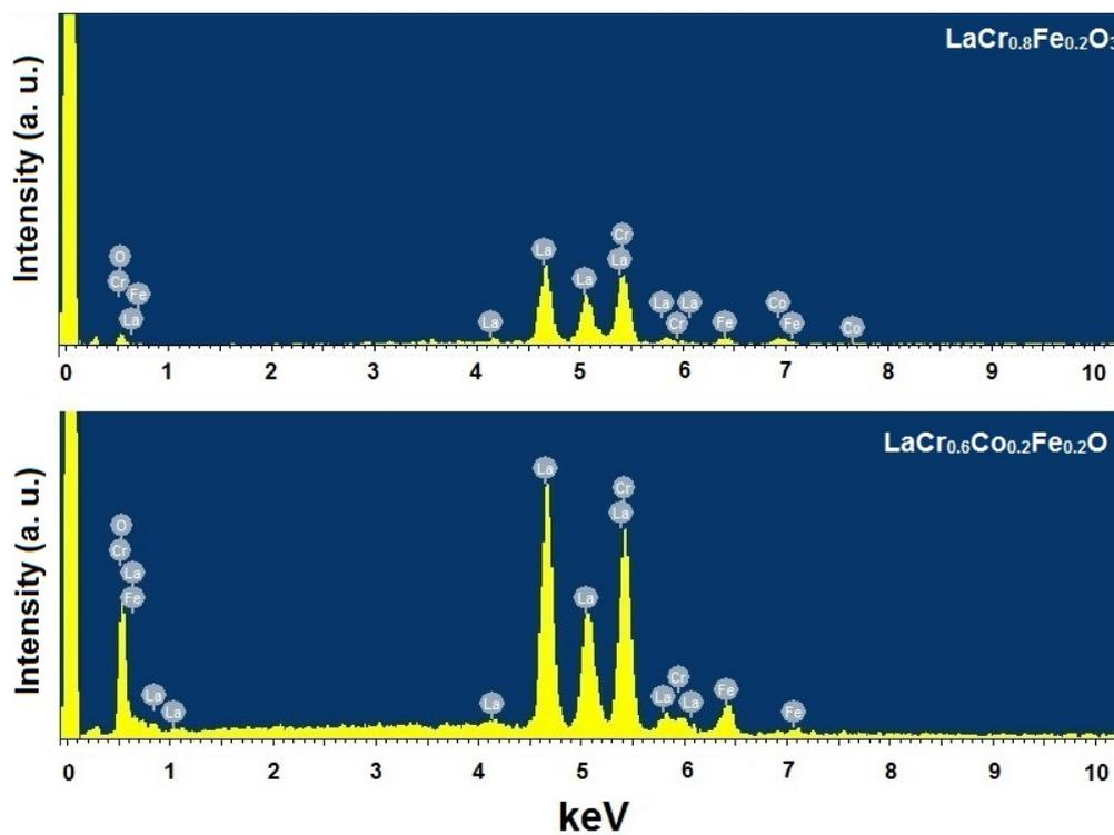
**Figure 3.** EDX analysis of LaCr<sub>0.8</sub>Fe<sub>0.2</sub>O<sub>3</sub> and LaCr<sub>0.6</sub>Co<sub>0.2</sub>Fe<sub>0.2</sub>O<sub>3</sub>.
