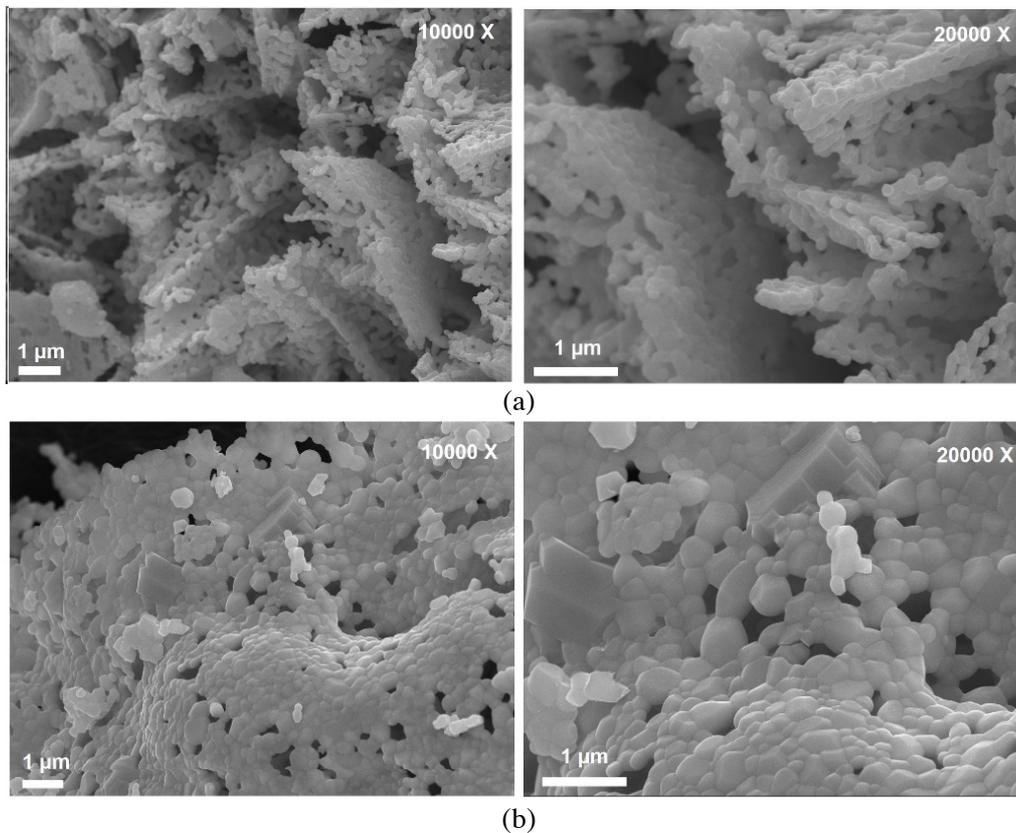
**Figure 2.** SEM images of (a) LaCr<sub>0.8</sub>Fe<sub>0.2</sub>O<sub>3</sub> and (b) LaCr<sub>0.6</sub>Co<sub>0.2</sub>Fe<sub>0.2</sub>O<sub>3</sub> to different magnifications.
