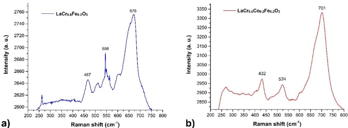
**Figure 5.** Raman shift of (a)  $\text{LaCr}_{0.8}\text{Fe}_{0.2}\text{O}_3$  and (b)  $\text{LaCr}_{0.6}\text{Co}_{0.2}\text{Fe}_{0.2}\text{O}_3$ .
