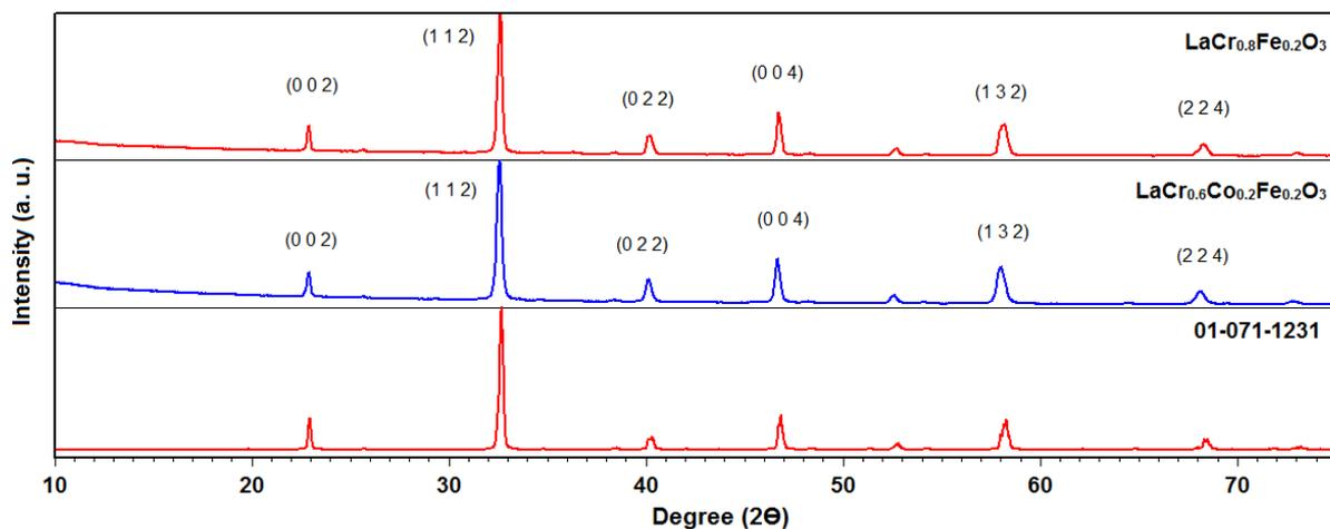
**Figure 1.** XRD patterns of  $\text{LaCr}_{0.8}\text{Fe}_{0.2}\text{O}_3$  and  $\text{LaCr}_{0.6}\text{Co}_{0.2}\text{Fe}_{0.2}\text{O}_3$  oxides.
