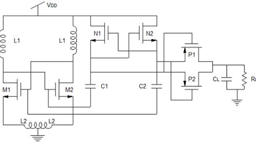
Figure 1. Single stage cross-coupled DC-DC converter with LC tank based oscillator.
