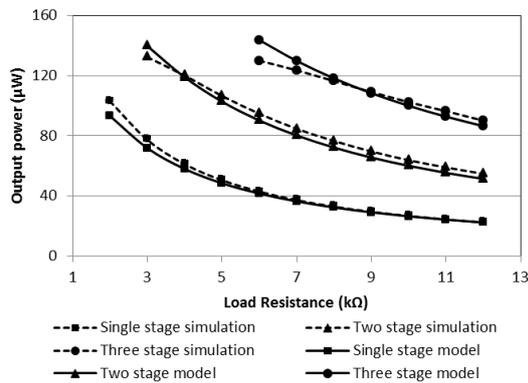
Figure 7. The variation of converter output power with load resistance for 1-3 stages.
