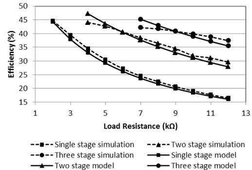
Figure 8. The variation of converter efficiency with load resistance for 1-3 stages.
