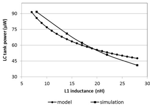
Figure 5. LC tank oscillator power consumption vs. L1 inductance.
