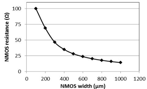
Figure 4. The variation of the NMOS resistance with MOSFET  $W$  ( $L=240$  nm).
