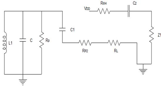
Figure 2. Equivalent half circuit model for Single stage DC-DC converter.
