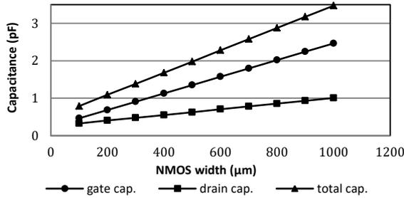
Figure 3. The variation of the NMOS capacitance with MOSFET width,  $W$  (length,  $L=240$  nm).
