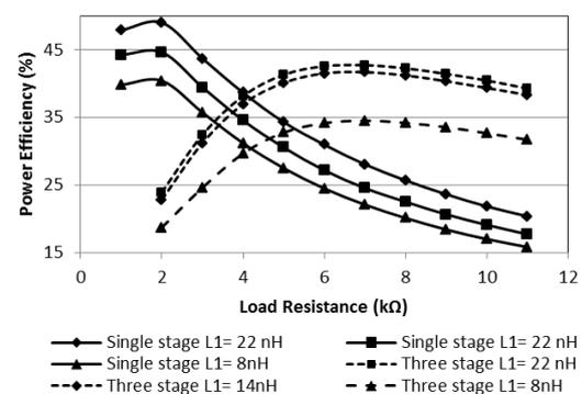
Figure 6. Converter power efficiency vs. load resistance and L1 size for 1 & 3 stages.
