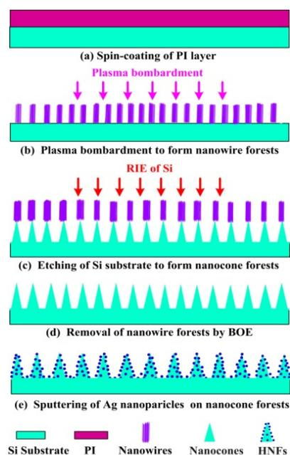
Figure 1. Fabrication process of the HNFs based on the PP technique.
