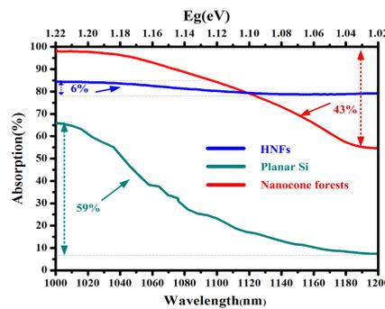
Figure 4. Absorption of the three Si-based structures in a wavelength range around the Si bandgap width (1000-1200nm).
