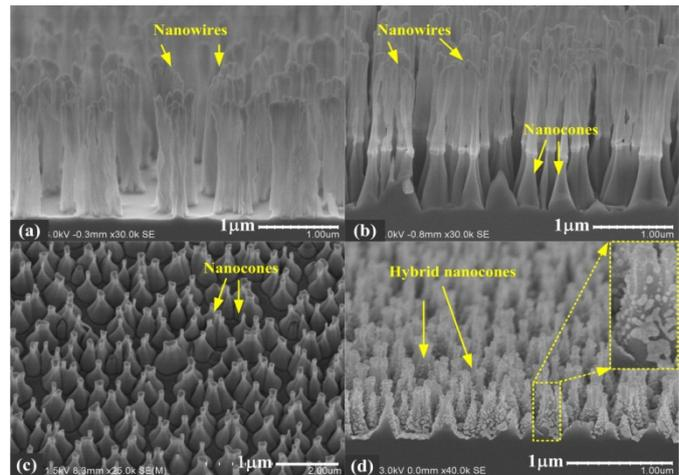
Figure 2. SEM images of nanostructure forests demonstrating formation process of the HNFs.
