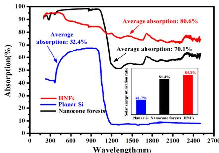
Figure 3. Average absorption and solar energy utilization ratio of planar silicon, nanocone forests and the HNFs.
