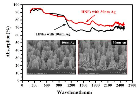
Figure 5. Absorption of HNFs with Ag nanoparticles of different sizes
