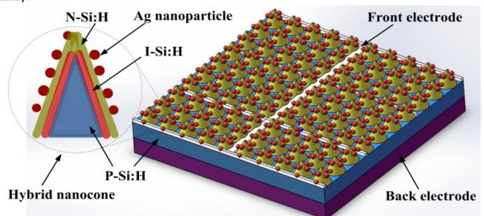
Figure 6. Schematic diagram of solar cells integrated with the HNFs.
