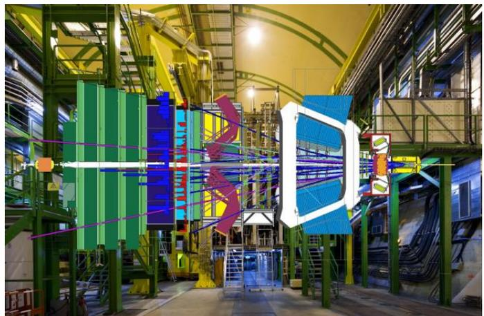
Figure 1. The LHCb forward spectrometer at the LHC with a sample event superimposed.
