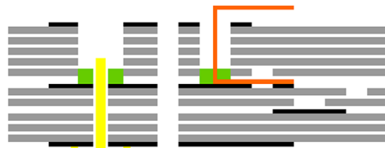
Figure 2. Schematic of the device's layers, with grey denoting individual or triplets of ceramic sheets, black metal patterns, green conductive adhesive, yellow an SMA connector, and orange metal wire.
