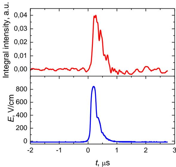
**Figure 1.** Optical response (red line) of the sample with double GaAs/AlGaAs QWs on the electric filed pulse (blue line) as an integral photodetector AC-coupled signal change with the analyser azimuth angle  $\alpha = +45^\circ$ .
