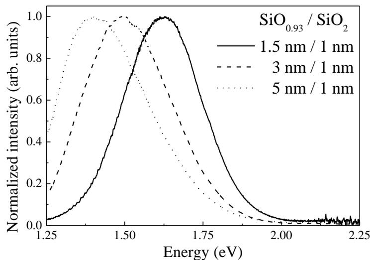
**Figure 1.** PL spectra of the SiO<sub>0.93</sub>/SiO<sub>2</sub> superlattices.
