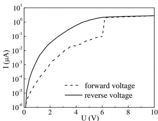
**Figure 4.** Current-voltage characteristic of the sample SN-2.
