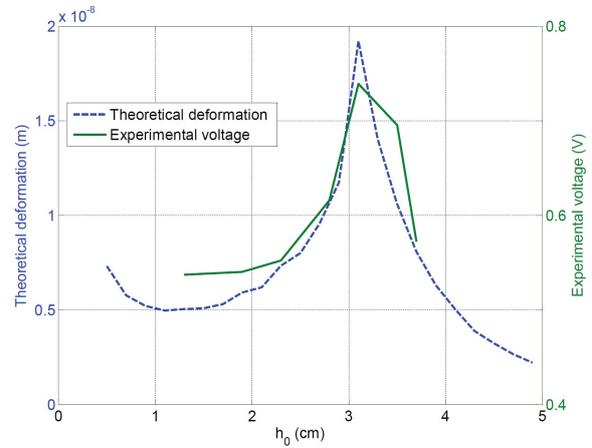
**Figure 3.** Theoretical deformation and experimental voltage for  $\theta = 45^\circ$  and  $\dot{\theta} = 0$
