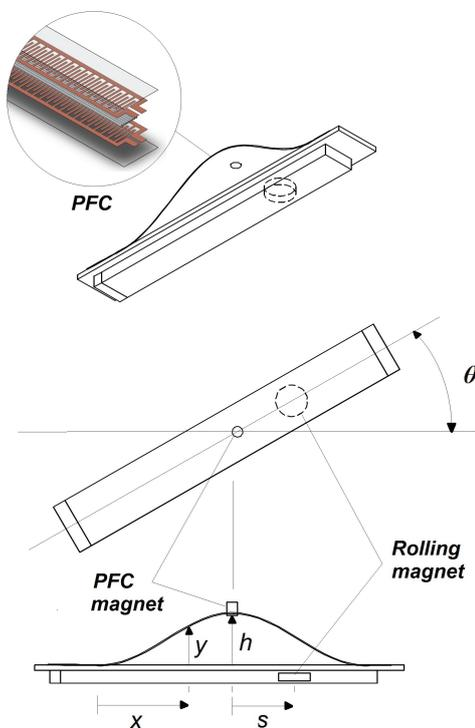
**Figure 1.** Schematic representation of the energy harvesting system
