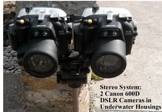
Figure 4. The stereo system used to capture the imagery.
