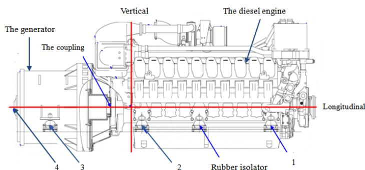
**Figure 9.** The structure schematic of the generating set.
