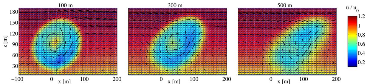
**Figure 6.** Streamwise (contours) and cross stream component (vectors) of the normalized simulated wind speed at different distances behind the wind turbine for the interval starting at 6:30 am.
