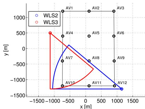
**Figure 1.** Layout of alpha ventus and position of the two lidars (WLS2, WLS3) that were used for the analysis and the scan area for measurements of the wake of AV10.
