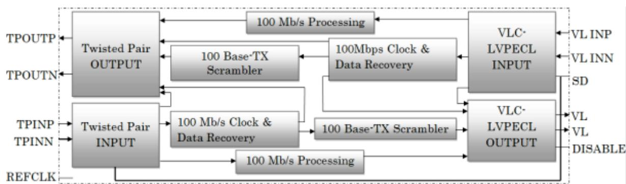
**Figure 1.** Ethernet to VLC transceiver.
