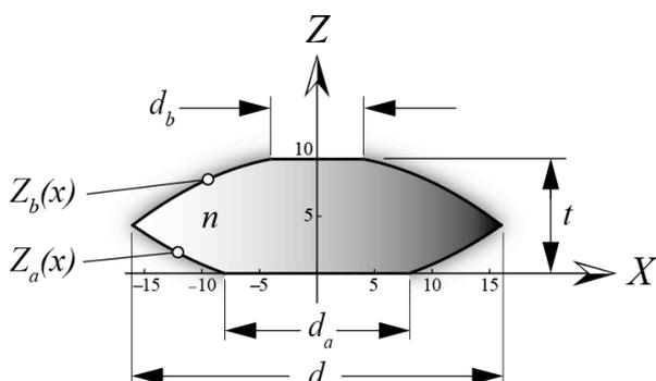
**Figure 2.** Here we show a catadioptric monolithic bi-flat bi-parabolic lens, with the parabolic sectors to be metalized with a thin layer of reflective metal, usually made of silver, aluminum, gold or platinum. The entrance window diameter corresponds to the diaphragm's diameter coupled to the first flat surface  $d_a = 16$  mm, the exit window diameter  $d_b = 8$  mm and the central thickness  $t = 10$  mm. The total diameter is  $d = 31.0179$  mm.
