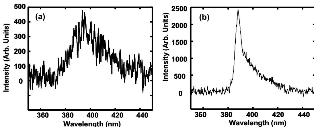
Fig. 4 Photoluminescence spectra. (a) for crystals shown in Fig. 1 (c), and (b) for lump crystals shown in Fig. 2 (a) that was taken from crystals in Fig. 1 (b) by laser brow-off.
