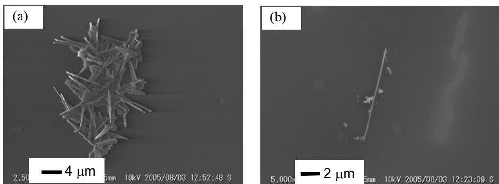
Fig. 2 ZnO nano-crystals taken out of the substrate shown in Fig. 1(c), by laser brow-off (a) and sonification (b).
