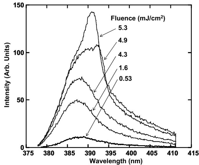
Fig. 3 Photoluminescence spectra as a function of pump fluence for nano-rods shown in Fig. 1 (a).
