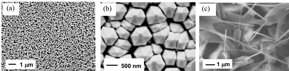
Fig. 1 SEM images of nano-structured ZnO crystals. (a) and (b) nano-rods crystals and (c) nano-wire pig-tailed micro crystals.
