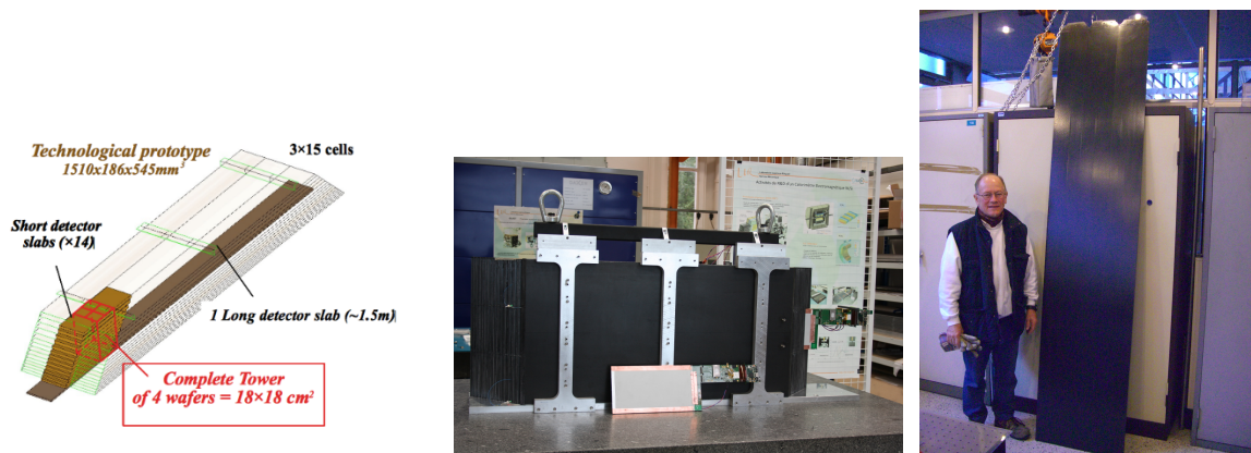
Figure 1. Left: Schematic view of the technological prototype with dimension. Center: Mechanical structure of the technical prototype with a short slab in front and one inserted on the right. Right: 2.5 m alveolar end-cap layer.
