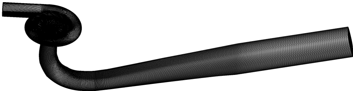
Figure 1. New grid (NG) with draft tube extension
