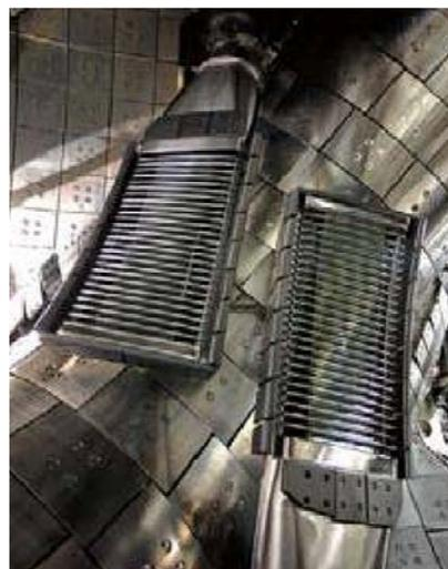
**Figure 1.** Phase controllable handshake shape-type antenna (HAS) installed in the LHD.
