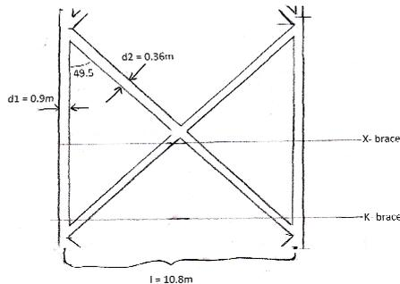
**Figure 2.** X- and K-brace positions shown on a side panel of the truss tower.
