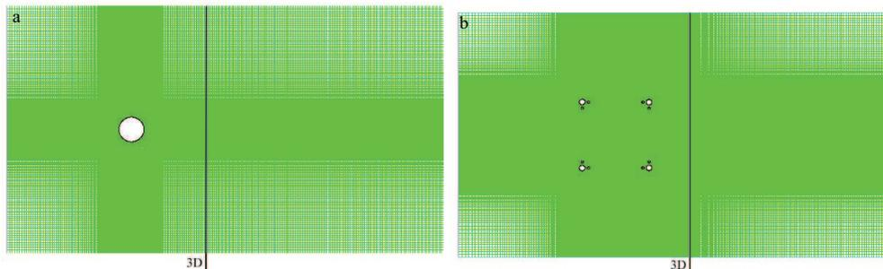
**Figure 1.** Grid for CFD simulations, line at 3D where rotor passes; monopile (left) and K-brace position for truss 0 degrees (right).
