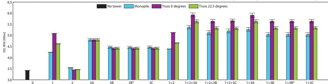
**Figure 6.** DEL on RFM behind monopile, truss 0 and truss 22.5 degree towers. Complexity of wind field increasing from left to right. All results presented at longitudinal resolution 25Hz and transversal and vertical grid resolutions 300 and 20 respectively, error bars showing standard deviation of the mean (details on wind field complexity components in Table 4).
