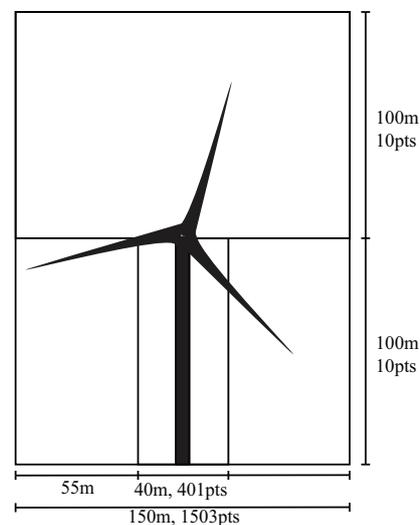
**Figure 3.** Wind field domain (fixed size) with maximum grid resolution, CFD domain at bottom centre (40m times 100m).
