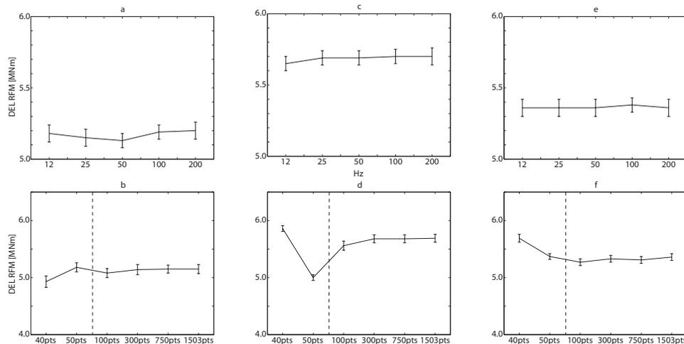
**Figure 5.** DEL for longitudinal (top) and lateral tower shadow resolutions (bottom). Left monopile tower, middle truss tower at 0 degrees and right truss tower at 22.5 degrees (dotted line show transition into interpolated turbulence).
