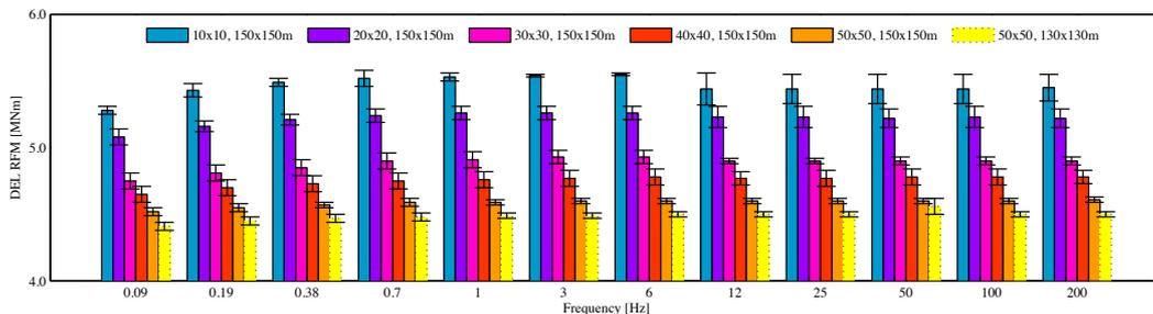
**Figure 4.** DEL on RFM with changing longitudinal and transversal resolutions for the wind field based on the one component Kaimal spectrum (no tower shadow present). Frequencies increase from 0.09Hz to 200Hz and grid point resolution from 10x10 to 50x50 points across domains of 150x150m and 130x130m.
