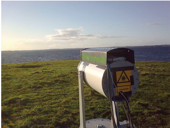
Figure 2. The scanning lidar measuring upwind towards the cliff of Bolund.
