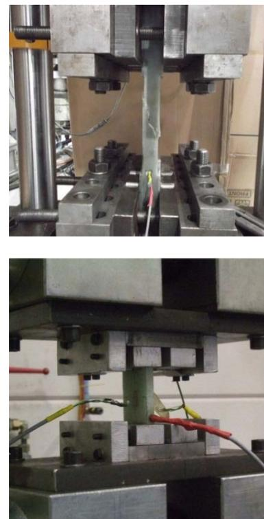
**Figure 5.** Top: S77 test configuration and failure mode. Bottom: S20 test configuration
