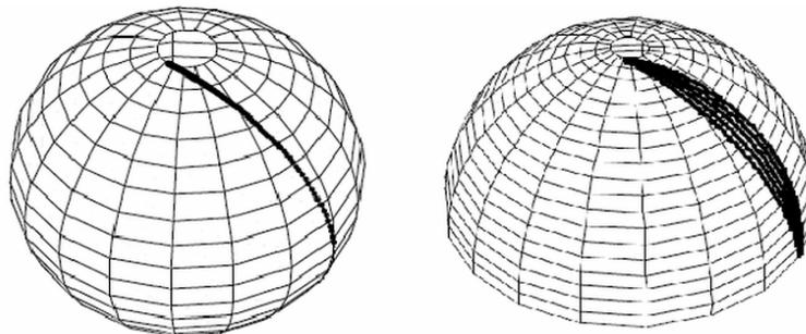
**Figure 1.** Geodesic path on a sphere (*left*) and semi-geodesic paths with different friction coefficients on a semi-sphere (*right*) [5]
