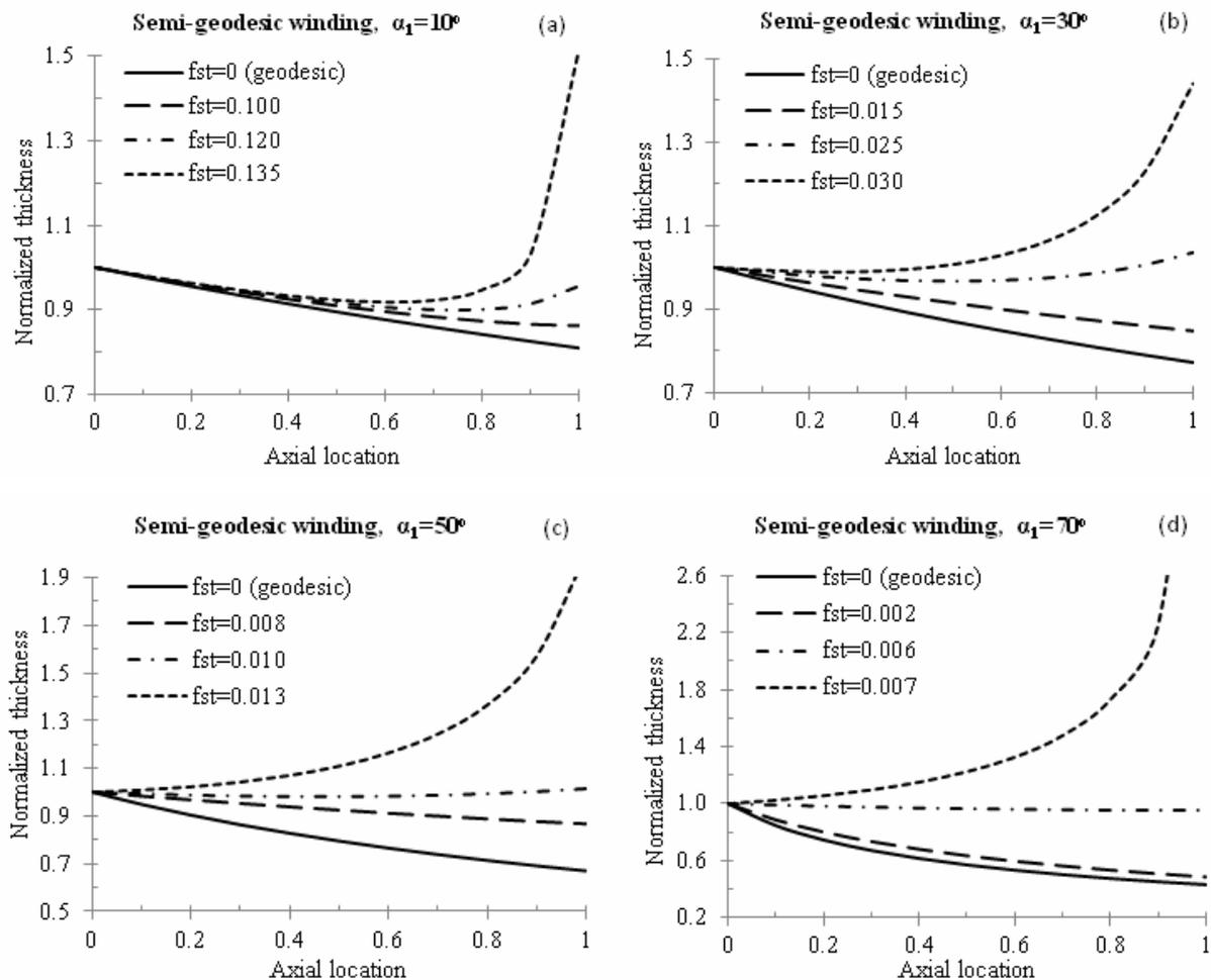
**Figure 4.** Effect of semi-geodesic winding on thickness for tower type 5 and initial winding angles (a)  $\alpha_1=10^\circ$ , (b)  $\alpha_1=30^\circ$ , (c)  $\alpha_1=50^\circ$ , (d)  $\alpha_1=70^\circ$ .
