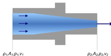
**Figure 4.** Schematic of the fluid flow through the conduit and the nozzle.
