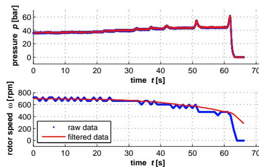
**Figure 13.** Transient response for hydraulic braking: the results from gradually closing the manual valve located before the nozzle (indicated in figures 6 and 7(b)).
