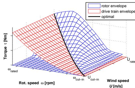
**Figure 5.** Operational envelopes of the rotor and hydraulic drive train assembly.
