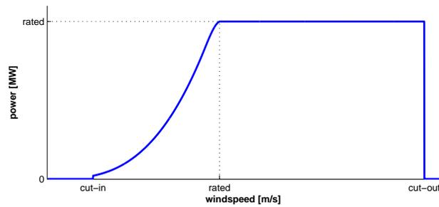
**Figure 2.** The conventional power curve of an arbitrary variable-speed, variable-pitch wind turbine.
