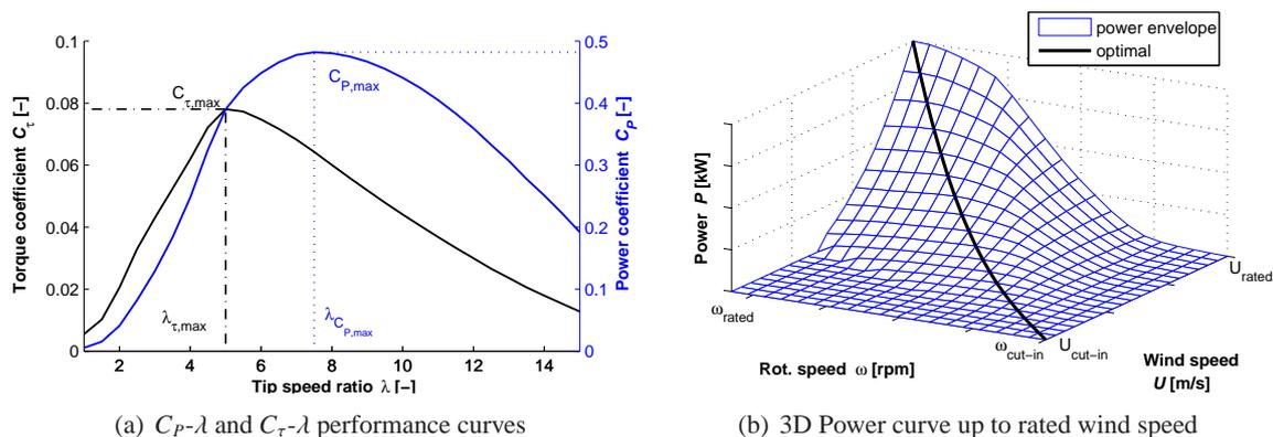
**Figure 3.** The aerodynamic performance of an arbitrary variable-speed wind turbine rotor at nominal pitch angle.
