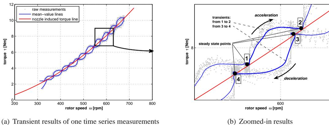
**Figure 10.** Steady state and transients explained for the torque-speed curve, corresponding to the time series with  $D_{nozzle} = 1.32\text{mm}$ .
