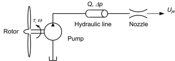
**Figure 1.** Simplified diagram of the proposed hydraulic transmission concept.
