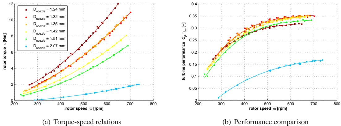
**Figure 9.** Steady-state results of the OJF measurements for different nozzles.
