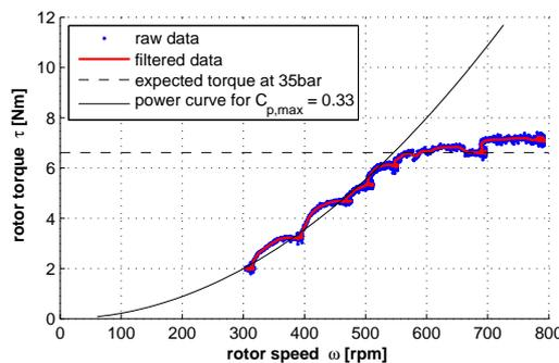
**Figure 12.** Transient response for drive train torque limitation using a pressure relief valve.
