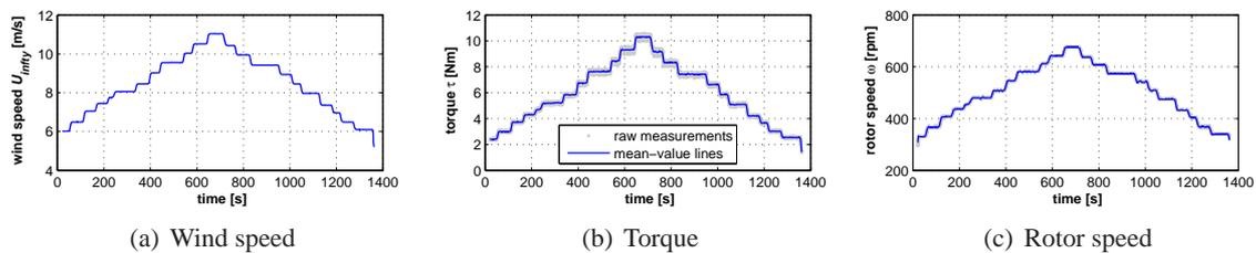
**Figure 8.** Time series for one continuous run of measurements; horizontal lines indicate steady state.
