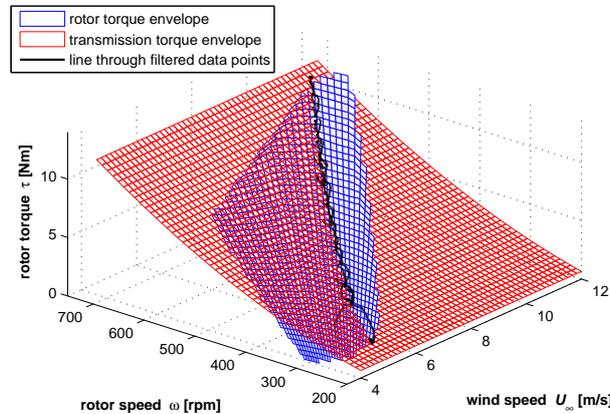
**Figure 11.** The measured transient response mapped onto the measured operational envelopes of the rotor and the fluid power transmission.
