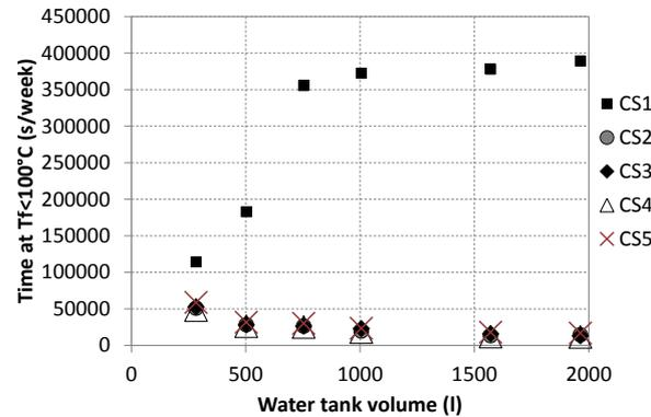
**Figure 9.** Total time flue gas temperature is below  $100^{\circ}\text{C}$  vs. water tank volume, for different strategies and 15 kW boiler.
