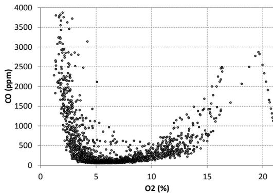
**Figure 1.** CO concentration in flue gas of a real pellet boiler as function of  $O_2$  concentration for the whole cycle (from start up to switch off). The optimal range of  $O_2$  is between 5% to 7%. [21]
