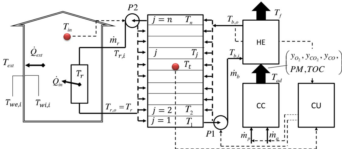
**Figure 3.** Scheme of the heating system modelled.
