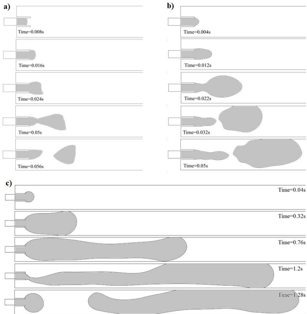
Figure 5: Bubble formation inside the minichannel inlet for different inlet conditions.
