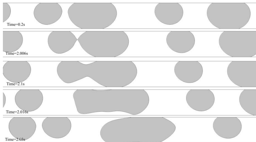
Figure 7: Bubble merging. (water u_{\max} = 1 \text{ ms}^{-1} , air u_{\max} = 3 \text{ ms}^{-1} )
