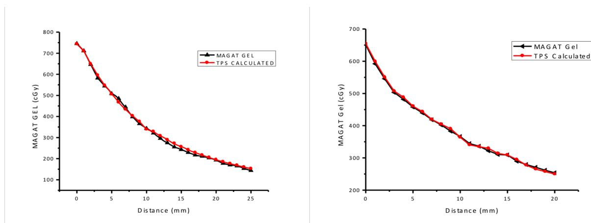
**Figure 3:** Comparison of MAGAT Polymer Gel with treatment planning system for (a) MammoSite<sup>®</sup> (b) Contura<sup>®</sup> balloon applicators
