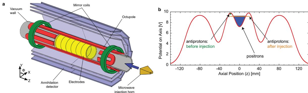
**Figure 1.** (a) Cut-away, drawing of the  $\bar{\text{H}}$  synthesis and trapping region. The superconducting atom-trap magnets, the annihilation detector, and some of the Penning-Malmberg trap electrodes are shown. An external solenoid (not shown) provides a 1-T magnetic field for the Penning-Malmberg trap. (b) The electrical potentials used for merging cold  $\bar{p}$  and positrons to make cold  $\bar{\text{H}}$ . See text for details.
