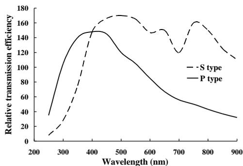
**Figure 2.** Relative transmission efficiency of a diffraction grating spectrometer for light polarized parallel (P) and perpendicular (S) to the grating lines.
