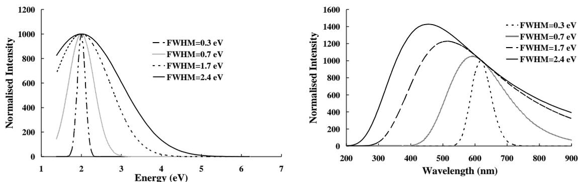
**Figure 3.** Equivalent wavelength and energy plots of a set of Gaussian luminescence bands centred at the same photon energy but different FWHM values
