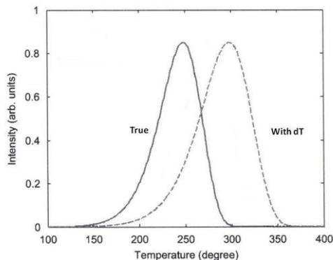
**Figure 1.** The solid line shows a true glow curve of a sample heated at 50 degrees per second and the dashed line is typical of recorded data based on the thermocouple temperature of the heater strip. The thermal gradient across the insulating sample introduces a variable lag of  $dT$  which is  $\sim 50$  degrees at the peak value in this example.
