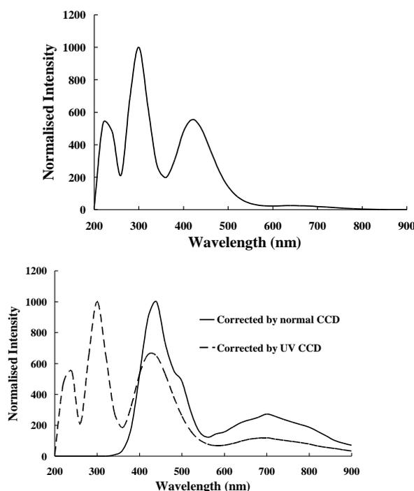
**Figure 4.** The spectra that would initially be collected by a spectrometer and PM tube (left) and the same signal as sensed by two different types of CCD detector (right). Note that after spectrometer correction and
