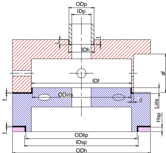
Fig.1: Details of different brazing joints in photocathode gun brazed in first cycle.
