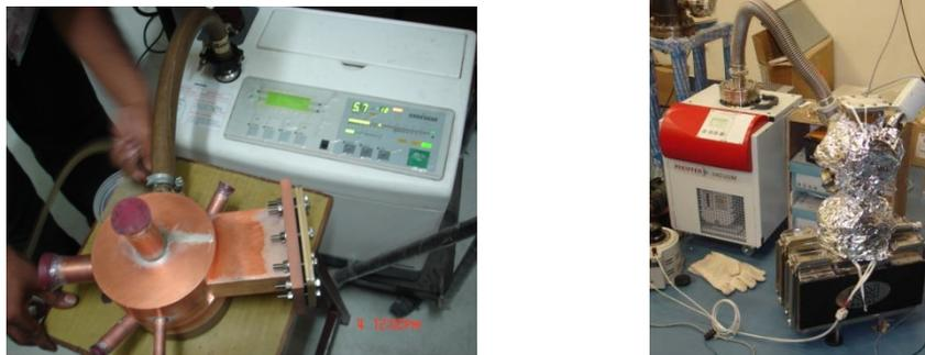
Fig.6: Photocathode RF gun being leak tested, and on the vacuum test setup
