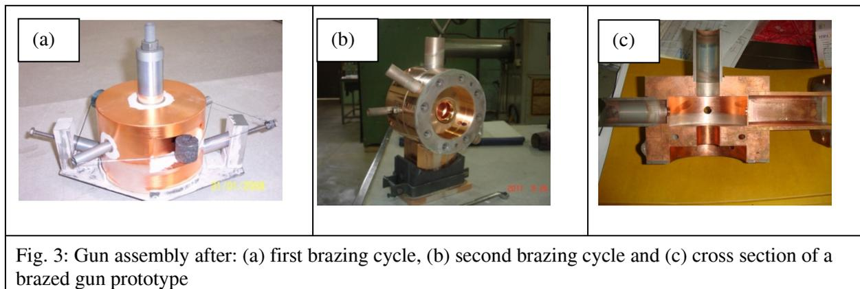
Fig. 3: Gun assembly after: (a) first brazing cycle, (b) second brazing cycle and (c) cross section of a brazed gun prototype
