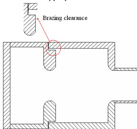
Fig. 5: Brazing clearance between the full-cell and half-cell
