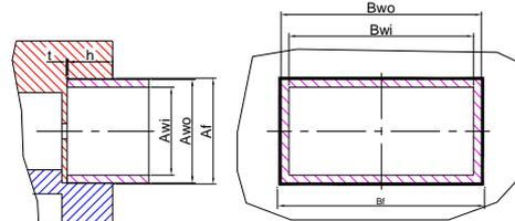
Fig. 2: Details of photocathode gun to waveguide brazing.
