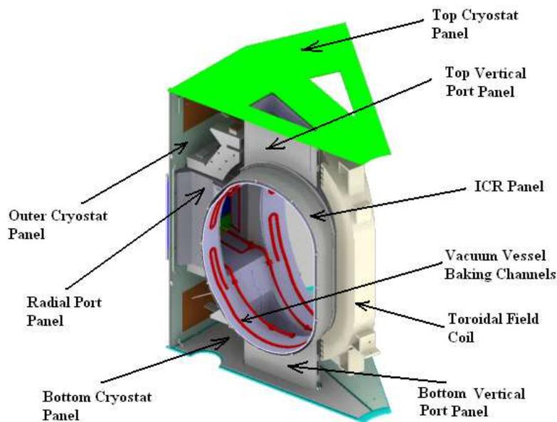
**Figure 1.** Schematics of SST-1 Tokamak with main sub-systems.
