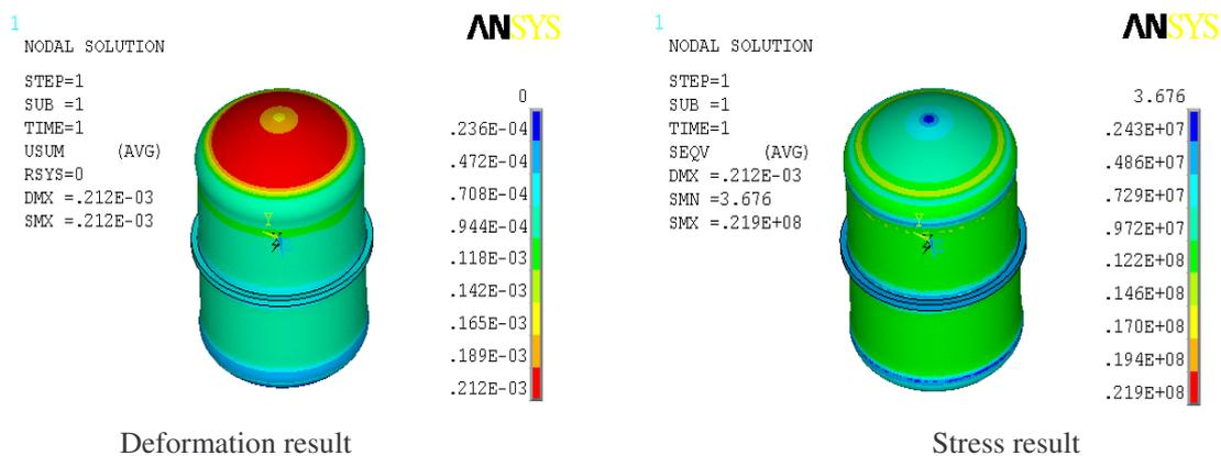
**Figure 2.** ANSYS results for deformation and stress values.
