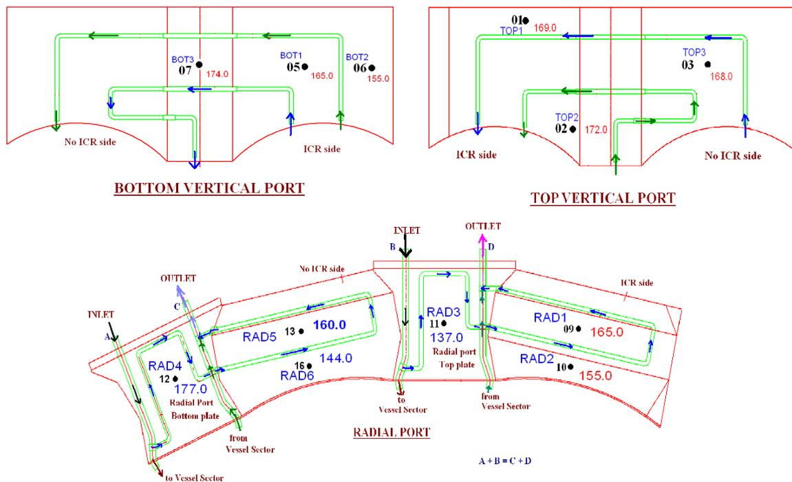
Figure 5. Temperature sensor locations of vertical and radial ports of one of the VM.
