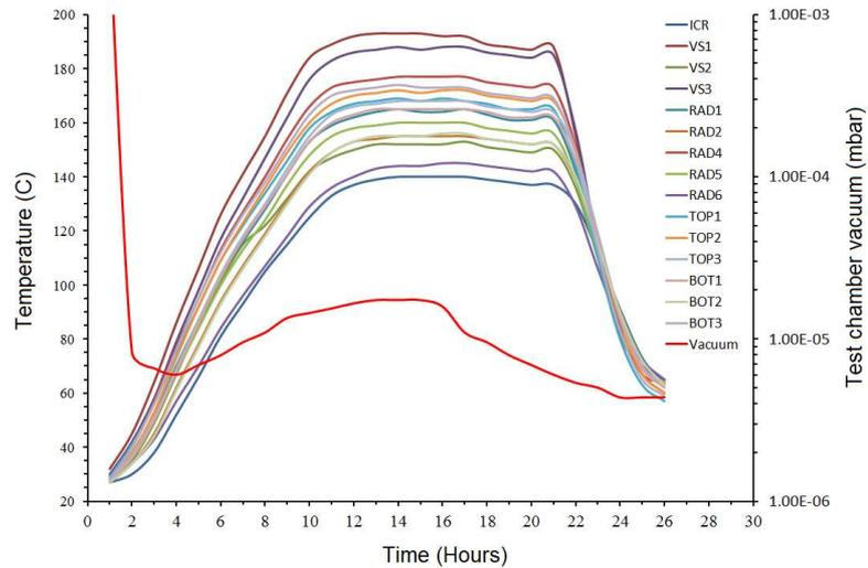
Figure 4. Test chamber pressure and temperature profiles of one of the VM.
