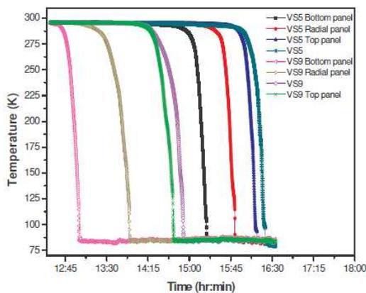
Figure 6. Vessel panels temperature with time.
