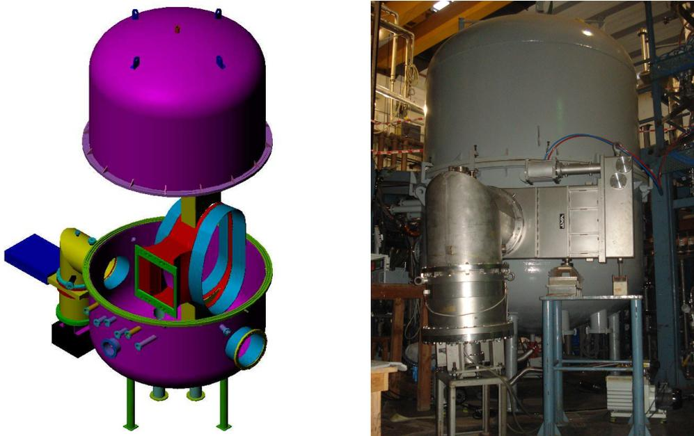
**Figure 3.** High vacuum chamber with vacuum accessories.
