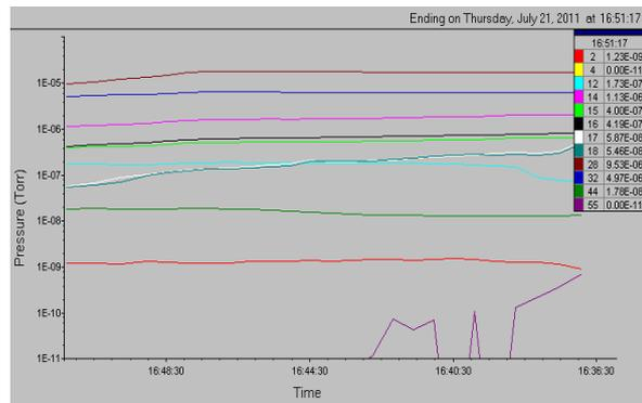
Figure 7. RGA Scan after cool down of shields.
