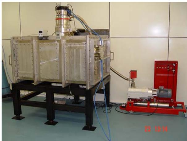
Fig. 3. Photograph of the chamber along with vacuum pumping system
