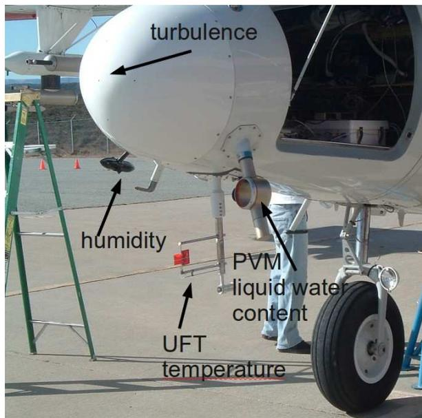
**Figure 1.** Radome of CIRPAS Twin Otter Research aircraft during POST. High frequency sensors measuring temperature (UFT), LWC (PVM), humidity and turbulence are closely co-located allowing to treat 40 Hz ( $\sim 1.4$  m spatial resolution) data as representative for the same sampling volume.
