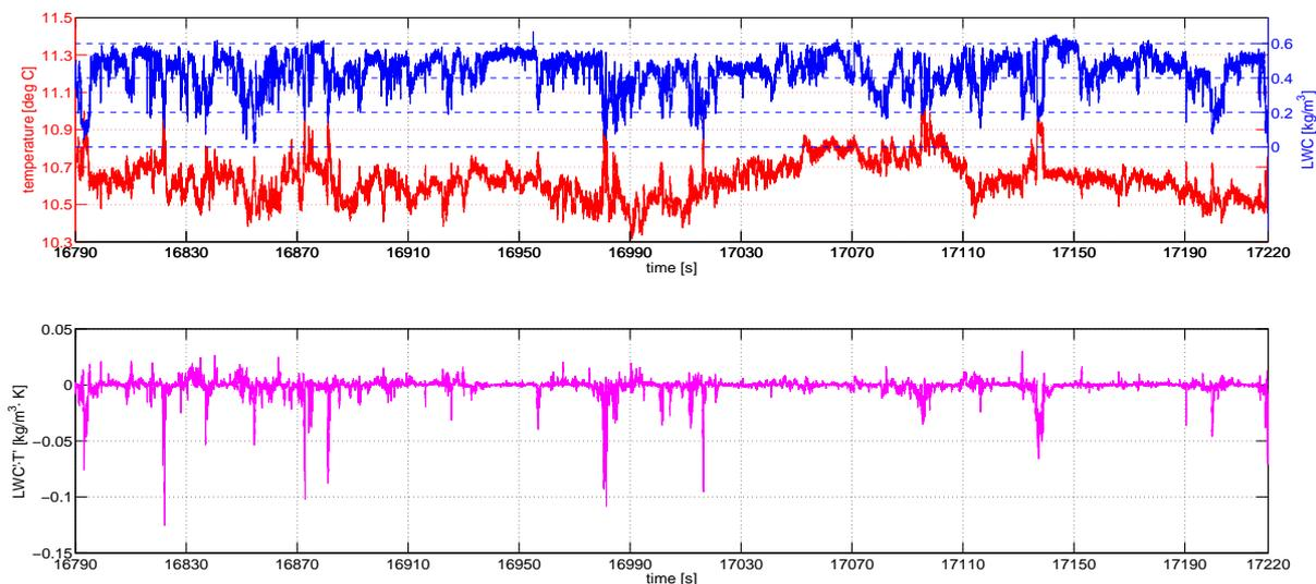
**Figure 7.** Upper panel: 100Hz (55cm spatial resolution) LWC and temperature record on a horizontal segment of TO13 flight inside the cloud deck. Lower panel: correlations of LWC a T fluctuations.
