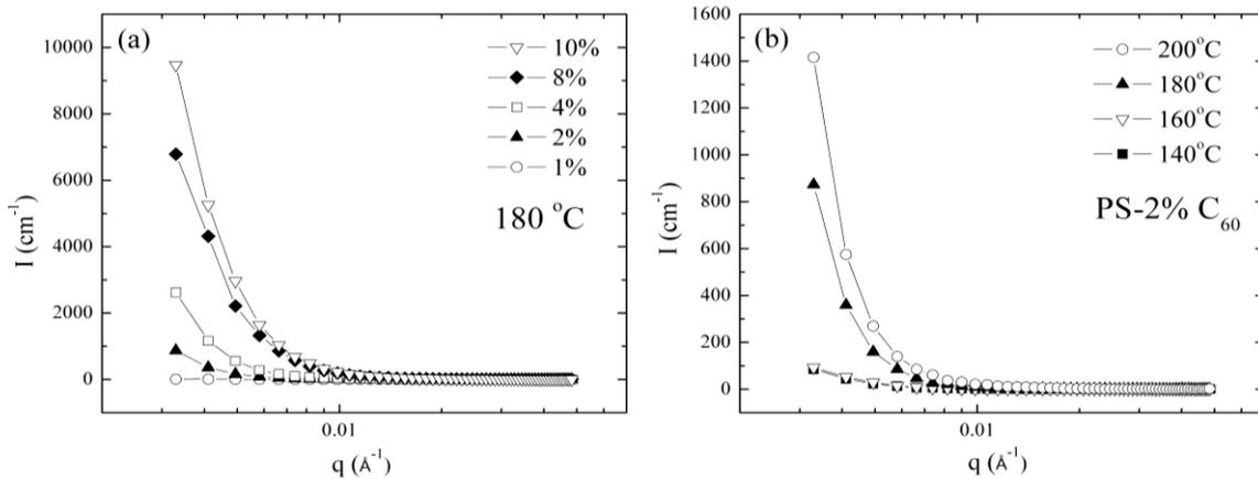
**Figure 2.** (a) SANS spectra of bulk polystyrene (PS) nanocomposites containing  $C_{60}$  mass fractions ranging from 1% to 10%, annealed at  $180^\circ\text{C}$  for constant time 14 min (b) effect of annealing temperature on PS-2%  $C_{60}$  at constant time 14 min.
