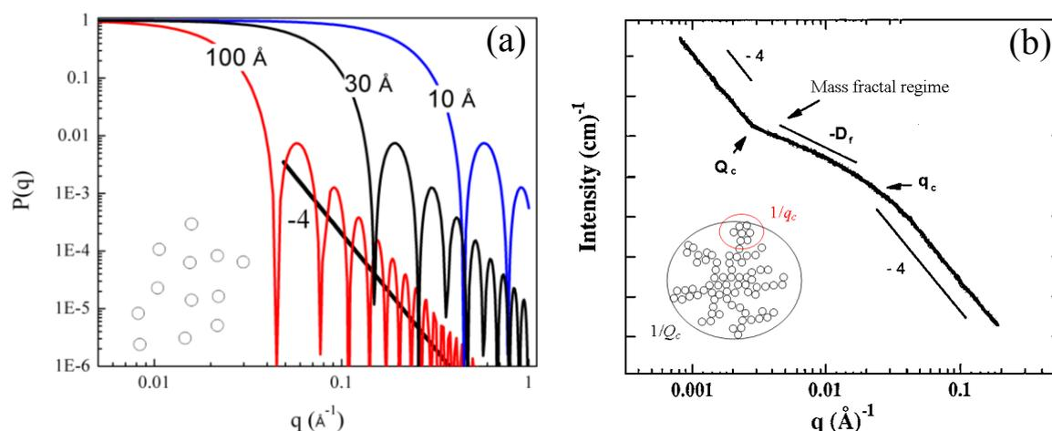
**Figure 5.** (a) Computed form factor of a sphere with radius  $r$  with respect to wavenumber  $q$ . Note the Porod regime towards high  $q$  value has  $-4 q$  dependence. (b) Typical scattering pattern from fractal system (See text below).
