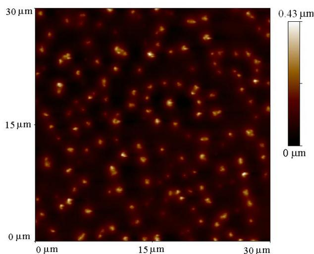
**Figure 8.** AFM topography scan of a representative PS- $C_{60}$  nanocomposite thin film ( $h = 135$ nm) annealed at  $180^\circ\text{C}$  for 30min.
