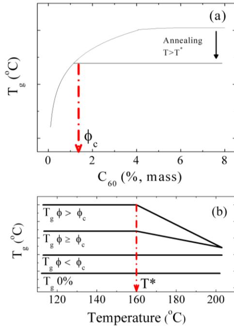
**Figure 3.** Schematics illustrating the effect of thermal annealing on the glass transition temperature ( $T_g$ ) of the nanocomposites as a function of (a)  $C_{60}$  loading and (b) annealing temperature. DSC agrees remarkably well SANS in determining agglomeration threshold  $\phi_c$  and  $T^*$ .
