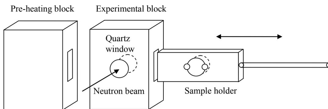
**Figure 1.** Schematic of the ‘Temperature Jump’ neutron kinetics scattering cell, depicting the pre-heating and experimental ovens and motorised sample holder. [18]
