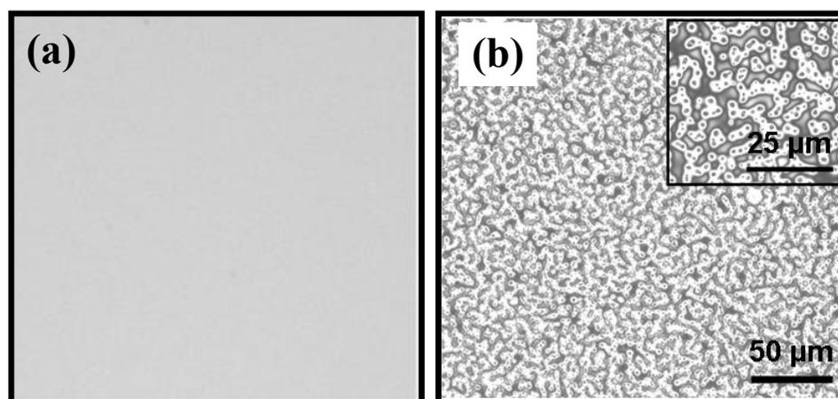
**Figure 7.** Optical micrograph of (a) neat PS and (b) PS thin film containing 5% mass fraction of  $C_{60}$  (thickness [h] = 150 nm) after annealing for 30 min at 180°C. Upon annealing, the neat film remains uniform while the filled counterpart shows a spinodal clustering morphology, reported in [16].
