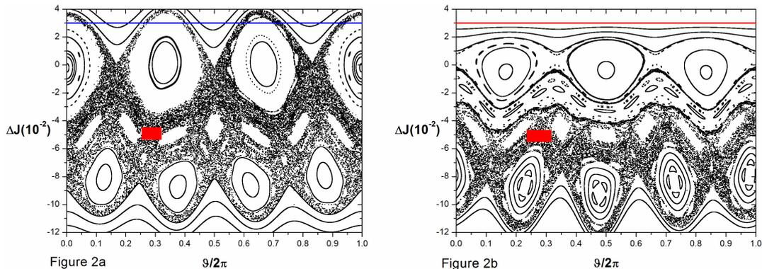
**Figure.2.** Poincaré sections for the resonant modes (1:3) and (1:4) with  $\alpha=0$  for: **(a)** Twist map, Eq. (4), without RT with  $\beta = -6.0 \times 10^{-4}$  and  $\eta = 2.99 \times 10^{-4}$ , the blue line at  $\Delta J=3$  is only to guide the eyes, it is not a RT. **(b)** Twist map, Eq.(5), with RT (in red) at  $\Delta J=3$ , with  $\beta = -7.5 \times 10^{-3}$  and  $\eta = 8.2 \times 10^{-3}$ .
