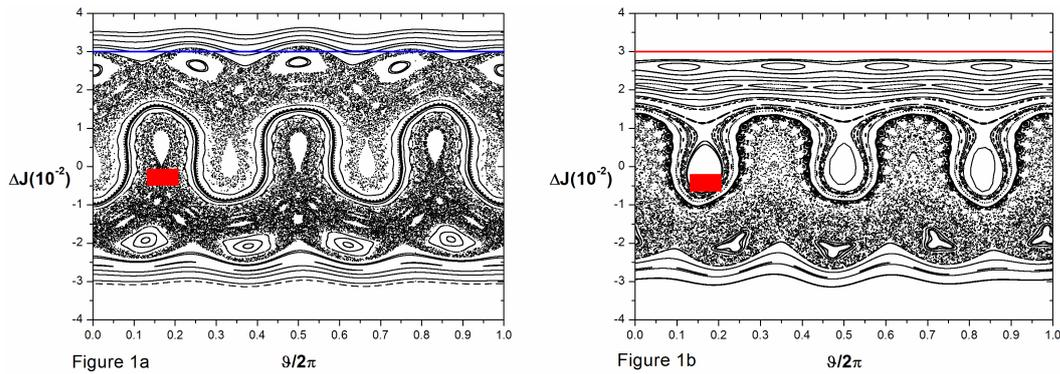
**Figure.1.** Poincaré sections for the resonant modes (1:3) and (1:4) for  $\alpha=160.15$ : **(a)** Non-twist map, Eq. (4), without RT with  $\beta = -1.3 \times 10^{-4}$  and  $\eta = 1.15 \times 10^{-4}$ , the blue line at  $\Delta J=3$  is only to guide the eyes, it is not a RT; **(b)** Non-twist map, Eq. (5), with RT (in red) at  $\Delta J=3$ , with  $\beta = -4.0 \times 10^{-3}$  and  $\eta = 9.2 \times 10^{-3}$ .
