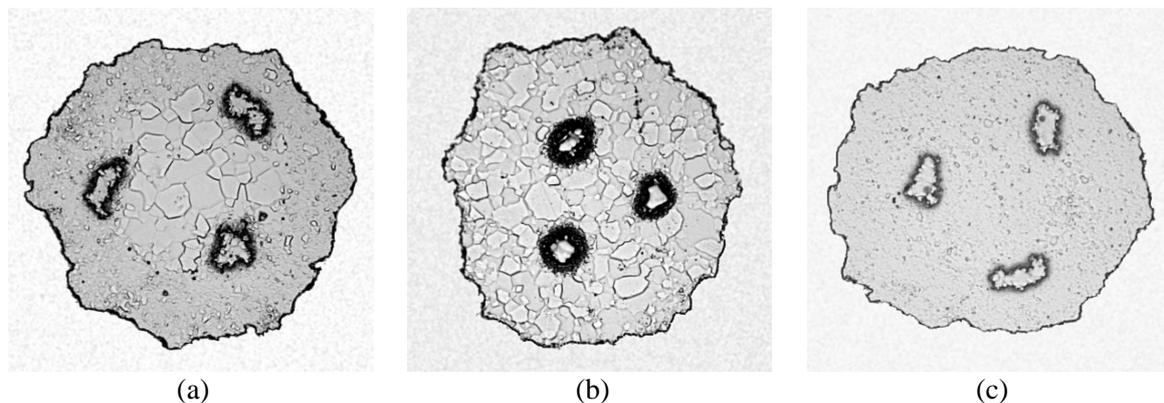
**Figure 6.** Filament restacks in subelements after recrystallization heat treatment: a – for ITS01-08 strand; b – for ITS02-08 strand; c – for ITS15-08 strand.
