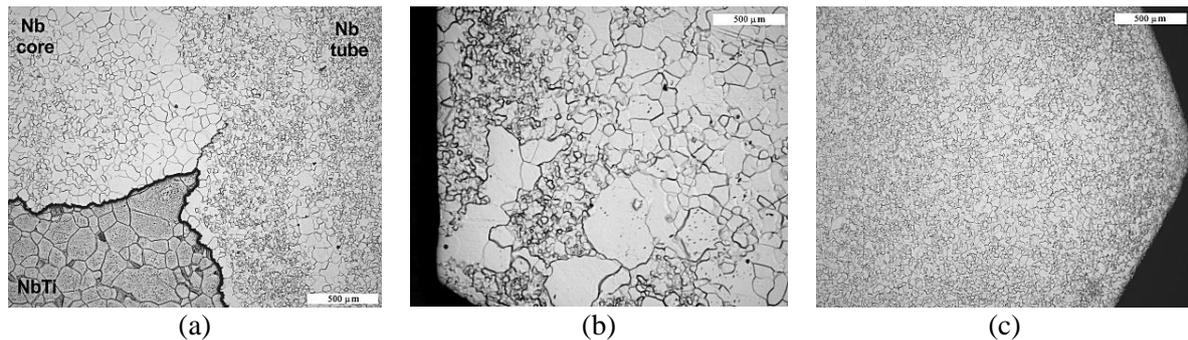
**Figure 5.** Nb elements after recrystallization heat treatment: a – for ITS01-08 strand; b – for ITS02-08 strand; c – for ITS15-08 strand.
