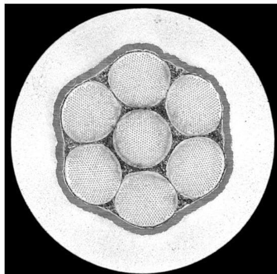
**Figure 3.** Final strand restack layout.
