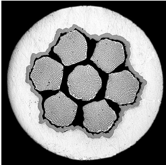
**Figure 4.** Typical cross-section of IT superconducting strand (0.82 mm in dia) formed from round multifilamentary subelements covered by tin layers.
