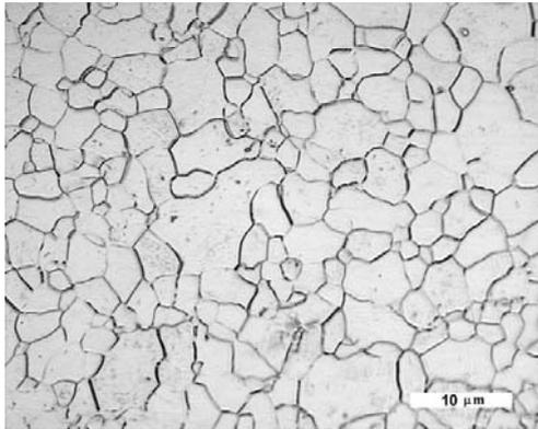
**Figure 7.** Nb grain structure in subelement filament of ITS15-08 strand.
