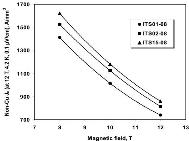
**Figure 10.** Non-Cu critical current density as a function of magnetic field for IT strands.
