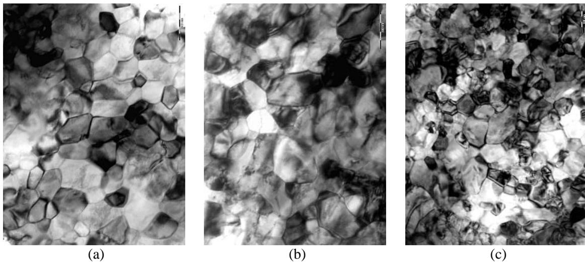
**Figure 9.** Grain structure of Nb<sub>3</sub>Sn in IT strands after reaction heat treatment: a – in ITS01-08 strand; b – in ITS02-08 strand; c – in ITS15-08 strand.
