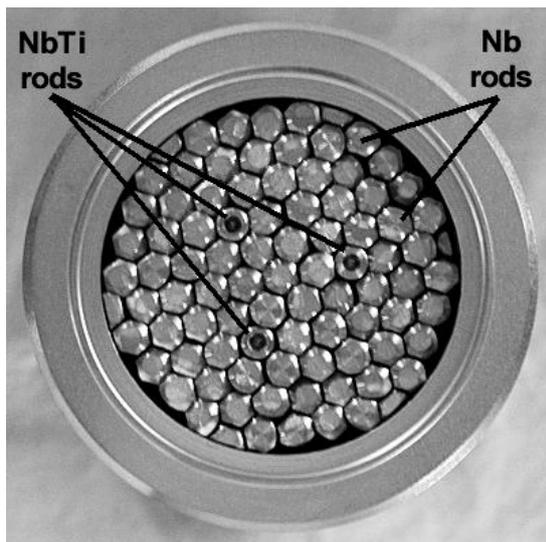
**Figure 2.** Filament composite billet design.
