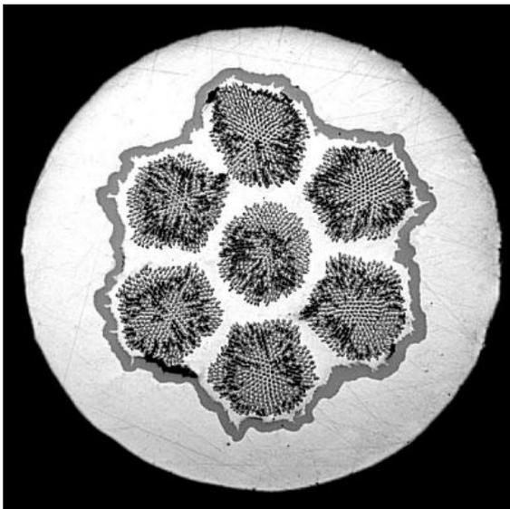
**Figure 8.** Typical cross-section of IT superconducting strand (0.82 mm in diameter) formed from round multifilamentary subelements after reaction heat treatment.
