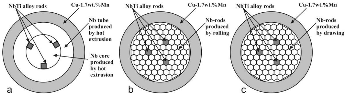
**Figure 1.** Formation of the initial composite billets for fabrication of composite filaments of advanced IT Nb<sub>3</sub>Sn superconducting strands: a – made from Nb tube and Nb core produced by hot extrusion; b – made from Nb rods produced by cold rolling process; c – made from Nb rods produced by cold drawing process.
