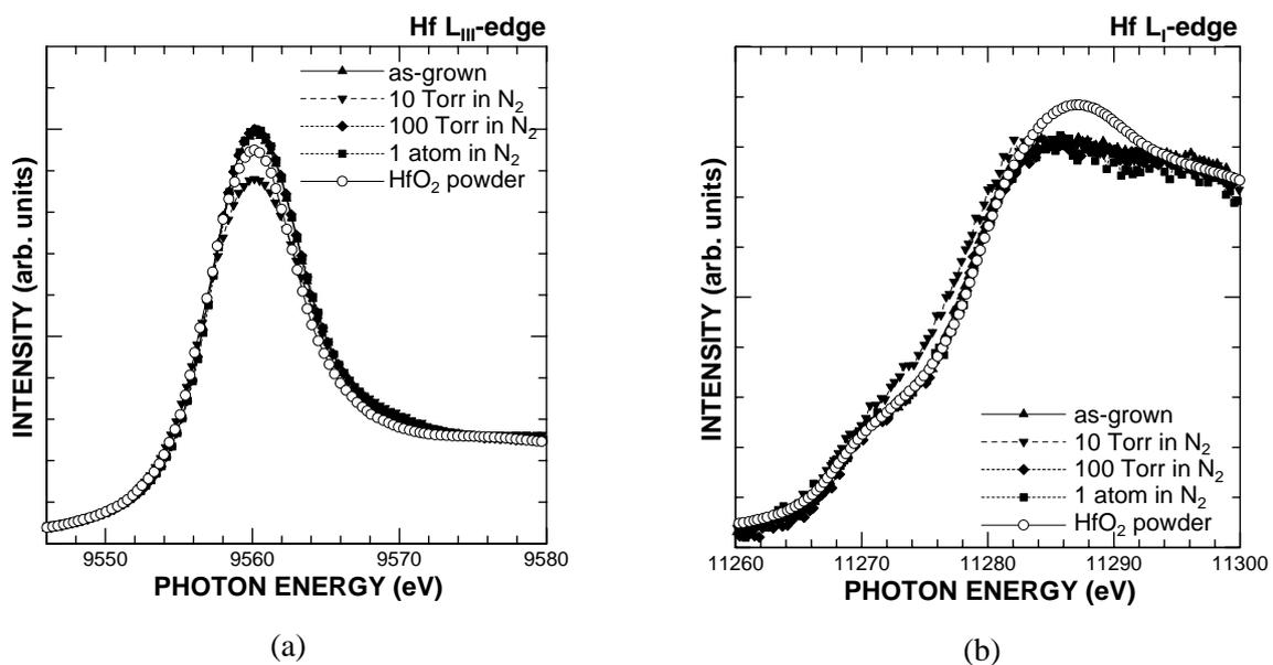
**Figure 1.** (a) Hf L<sub>III</sub>- and (b) Hf L<sub>I</sub>-edge XANES spectra for HfSiON films and HfO<sub>2</sub> powder.
