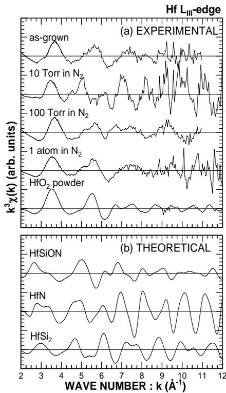
**Figure 2.** Hf L<sub>III</sub>-edge EXAFS oscillation functions  $k^3\chi(k)$  spectra for (a) HfSiON films and HfO<sub>2</sub> powder, and (b) theoretical EXAFS spectra for HfSiON, HfN, and HfSi<sub>2</sub>. Theoretical EXAFS spectra were generated by FEFF8. For the theoretical spectra, the Debye-Waller factor was assumed as 0.05 Å for the bond length below 4.0 Å and 0.075 Å for the bond length above 4.0 Å.
