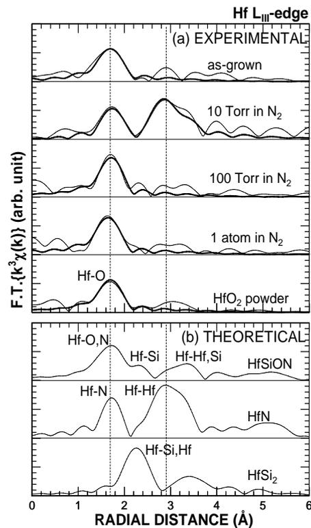
**Figure 3.** Fourier transform of Hf L<sub>III</sub>-edge EXAFS oscillation functions  $k^3\chi(k)$  spectra for (a) HfSiON films and HfO<sub>2</sub> powder (thin solid lines: experimental data, thick solid lines: curve-fitting data), and (b) theoretical EXAFS spectra for HfSiON, HfN, and HfSi<sub>2</sub>. The Fourier transformation was performed in the  $k$  range of 3.0 – 10.0 Å<sup>-1</sup>. Theoretical EXAFS spectrum was generated by FEFF8.
