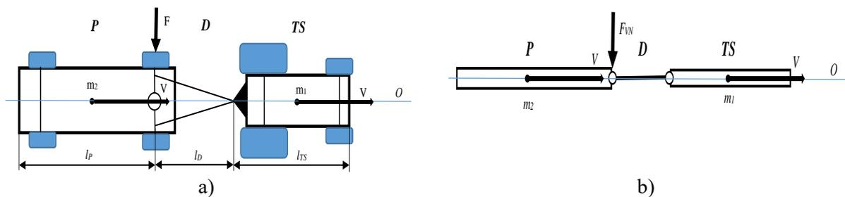
**Figure 1.** RT configuration (a) and simplified schematic of RT three-link mechanism (b). TS – traction truck, P – turntable trailer (PP), D – drawbar, FVN – external action,  $l_{TS}$ ,  $l_D$ ,  $l_P$  – length of the traction truck, drawbar and trailer,  $O$  – driving direction of RT,  $m$  – weight,  $V$  – speed of respective elements of RT.
