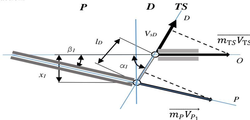
**Figure 3.** Condition for determining the maximum permissible external action. *TS* – traction truck, *P* – turntable trailer (*PP*), *D* – drawbar, *l<sub>D</sub>* – drawbar length, *x<sub>1</sub>* – value of lateral displacement of element *P*,  $\alpha_1, \beta_1$  – angles of axis displacement of elements *D* and *P* respectively from movement direction *O*,
